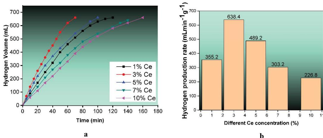
Fig. 4. Effect of Ce concentration on the hydrogen production in the presence of different Ce concentrations: (a) hydrogen volume vs. time and (b) hydrogen production rate vs. Ce concentration (%).
