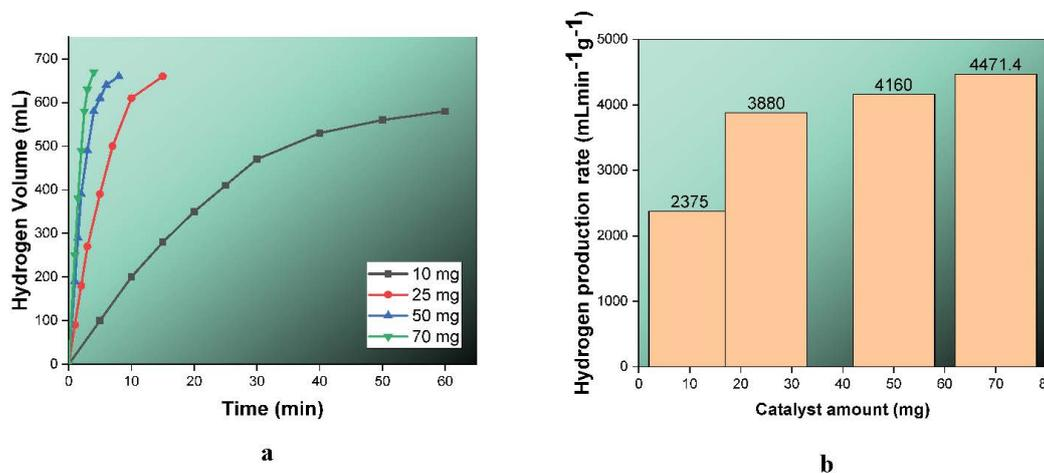
Fig. 7. Effect of catalyst amount on the hydrogen production in the presence of different Co-La-Ce-B catalyst amounts: (a) hydrogen volume vs. time and (b) hydrogen production rate vs. catalyst amount (mg).
