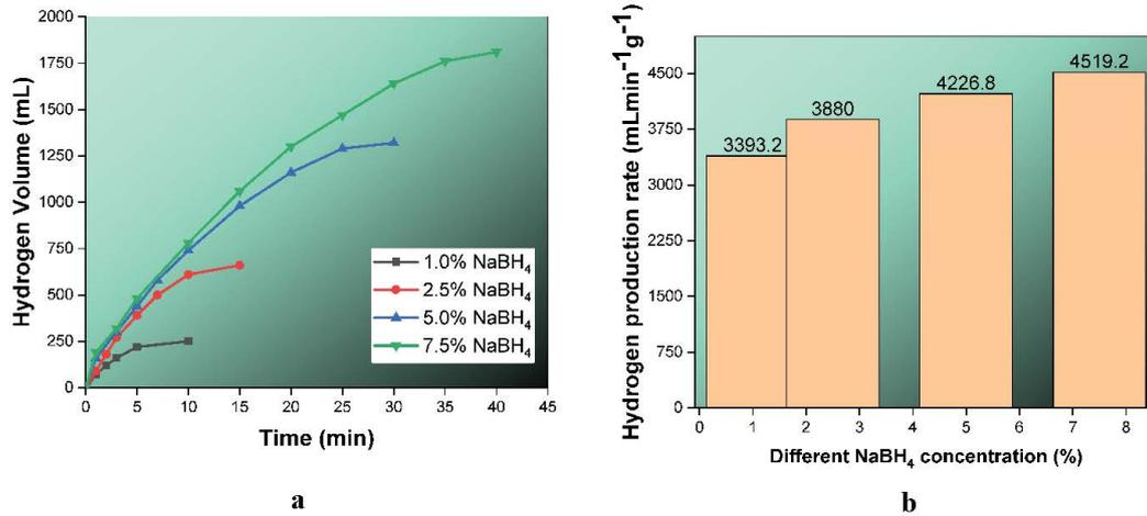
Fig. 6. Effect of NaBH<sub>4</sub> concentration on the hydrogen production in the presence of different NaBH<sub>4</sub> concentrations: (a) hydrogen volume vs. time and (b) hydrogen production rate vs. NaBH<sub>4</sub> concentration (%).
