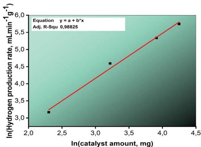
Fig. 13. The graph of ln(hydrogen production rate) vs. ln(catalyst).
