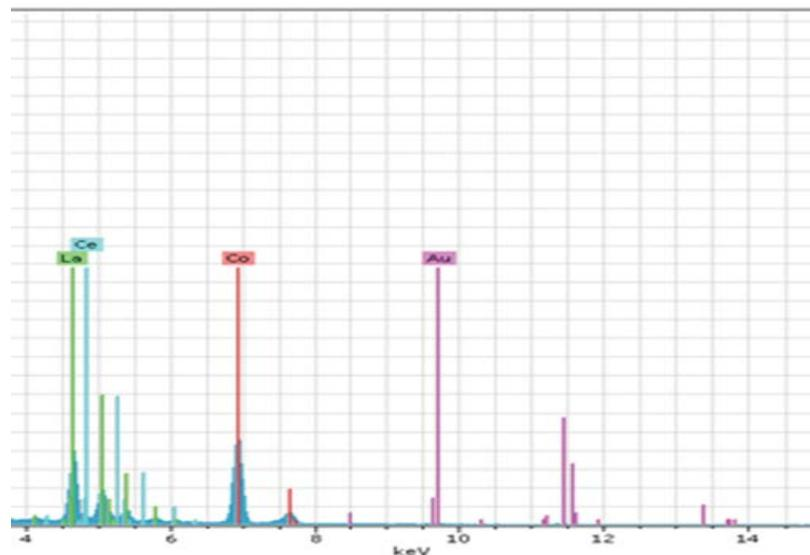
Fig. 2. EDX spectrum of Co-La-Ce-B catalyst.
