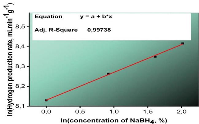
Fig. 11. The graph of ln(hydrogen production rate) vs. ln(NaBH<sub>4</sub>).
