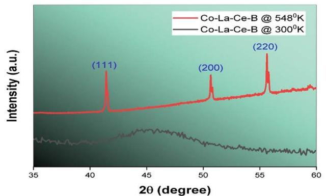
Fig. 3. XRD patterns of the Co-La-Ce-B catalysts heated at different temperatures: 300°K (black line) and 548°K (red line).
