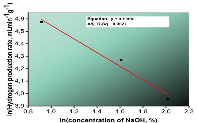
Fig. 12. The graph of ln(hydrogen production rate) vs. ln(NaOH).
