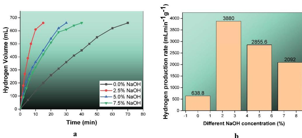
Fig. 5. Effect of NaOH concentration on the hydrogen production in the presence of different NaOH concentrations: (a) hydrogen volume vs. time and (b) hydrogen production rate vs. NaOH concentration (%).
