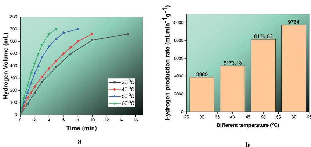
Fig. 8. Effect of temperature on the hydrogen production at different temperatures: (a) hydrogen volume vs. time and (b) hydrogen production rate vs. temperature (°C).
