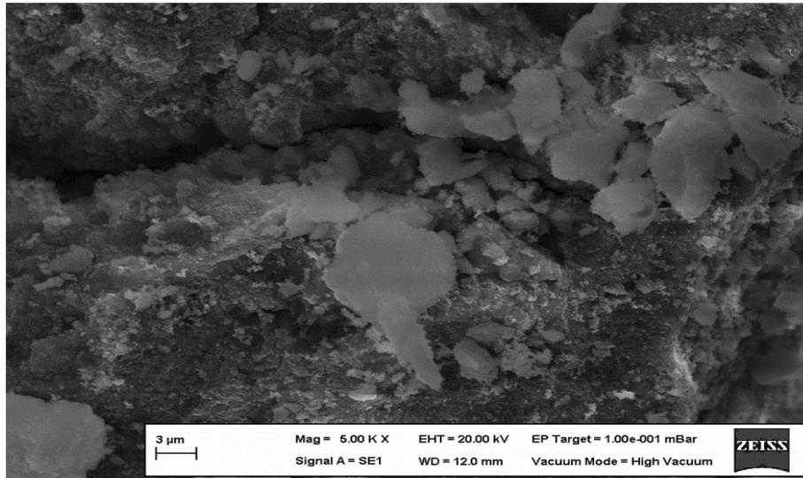
Fig. 1. SEM image of Co-La-Ce-B catalyst.
