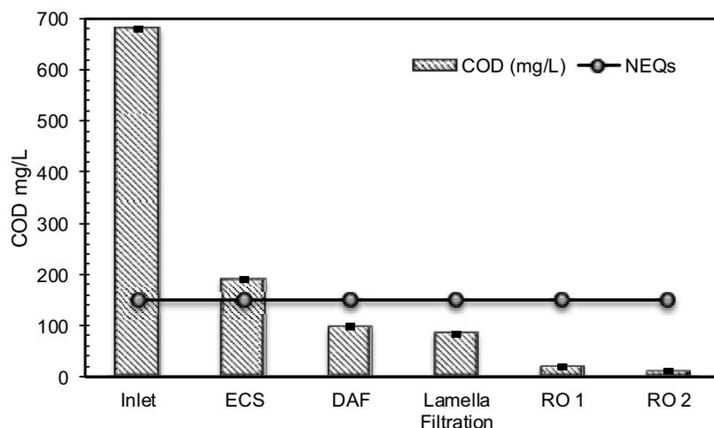
Fig. 10. Effect of COD (mg/L) of different components in ETP compared to NEQs.
