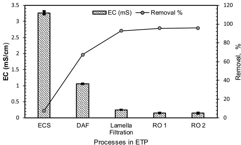
Fig. 7. Effect of EC (mS/cm) on textile dye-bath effluents.
