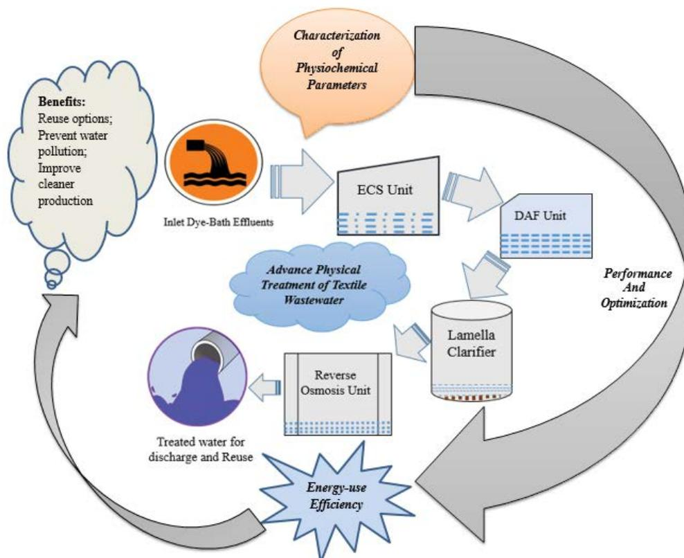
Fig. 1. Illustration of advanced physical treatment of textile dye-bath effluents including inlet raw water, electrocoagulation system (ECS), dissolved air flotation (DAF), lamella clarifier, reverse osmosis unit, treated water (temperature 25°C; initial pH: 12.38).
