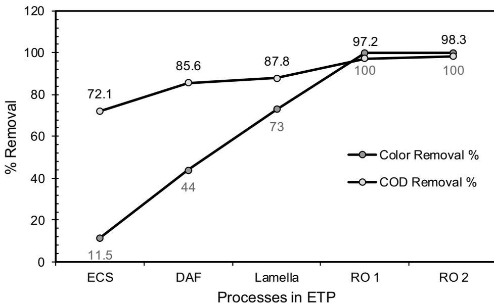
Fig. 11. Effect of COD and color on ETP processes of treated effluent.
