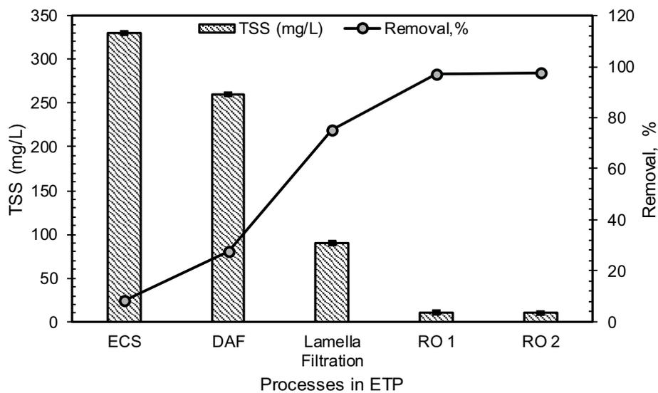
Fig. 8. The effect of TSS on textile wastewater.
