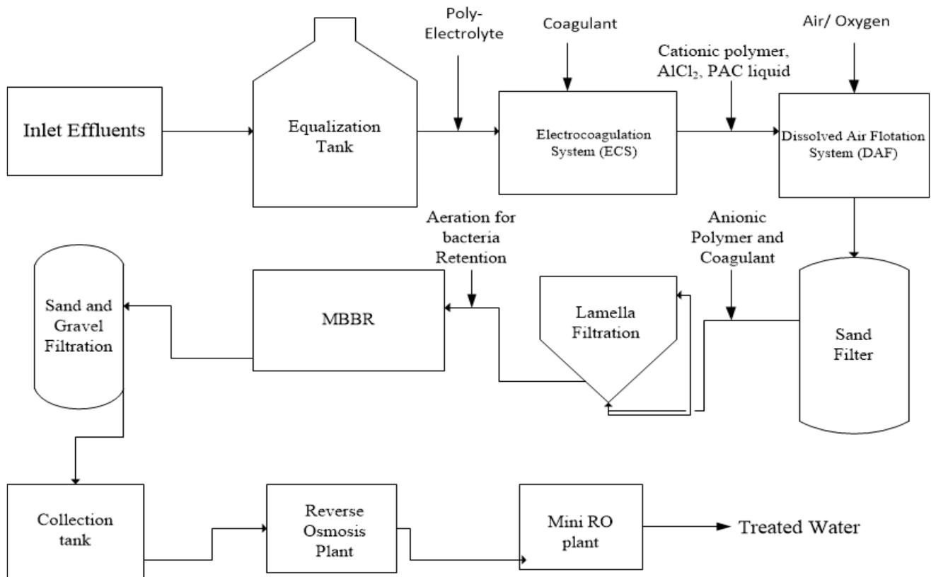
Fig. 2. Block diagram of the advanced system of the effluent treatment plant.
