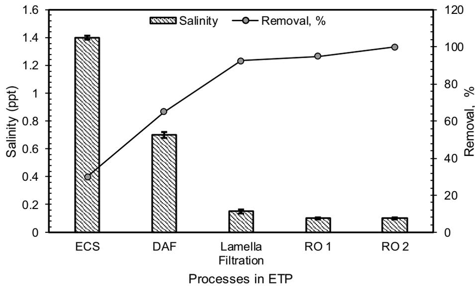
Fig. 6. Effect of salinity (ppt) in textile wastewater.
