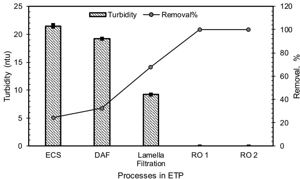
Fig. 5. Effect of turbidity on wastewater.
