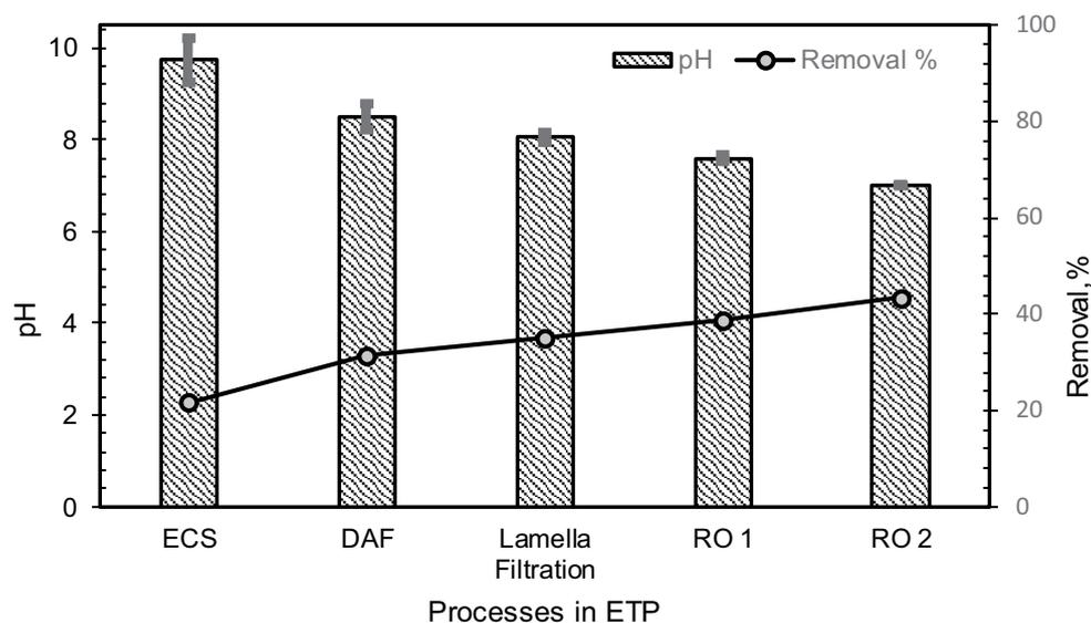
Fig. 3. Effect of pH on textile dye-bath effluents (temperature 25°C; initial pH: 12.38).
