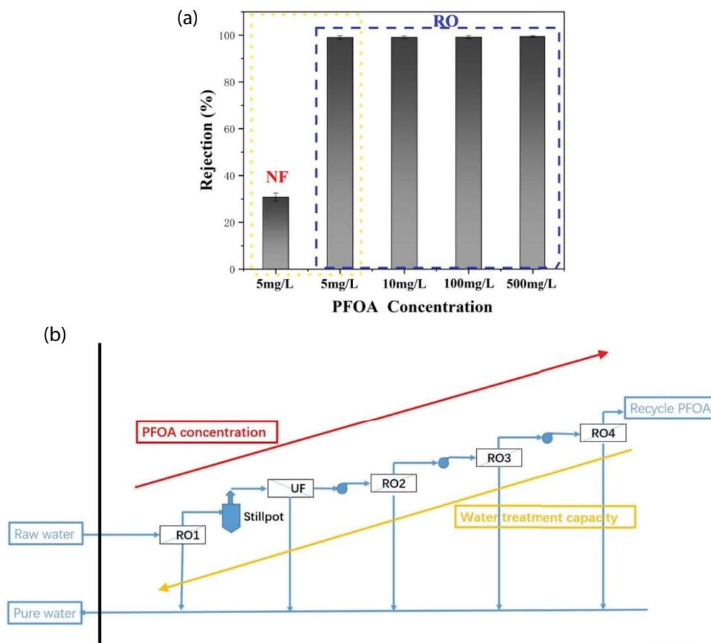
Fig. 1. The membrane rejection with different PFOA initial concentration (a), and the multi-stage RO unit technological process (b).
