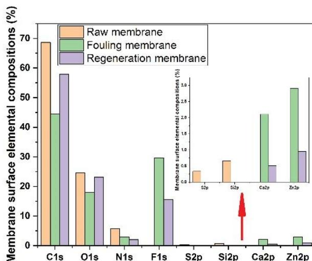
Fig. 3. Elemental surface compositions of raw membrane, fouling membrane, and regeneration membrane.
