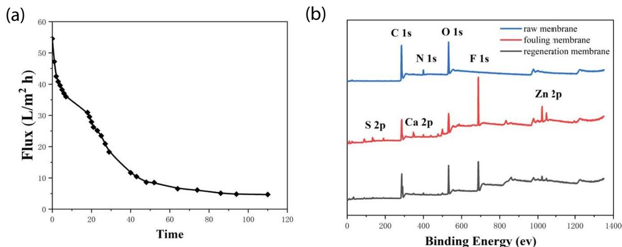
Fig. 2. The raw water flux of membrane (a), XPS wide spectra of origin membrane, fouling membrane and regeneration membrane (b).
