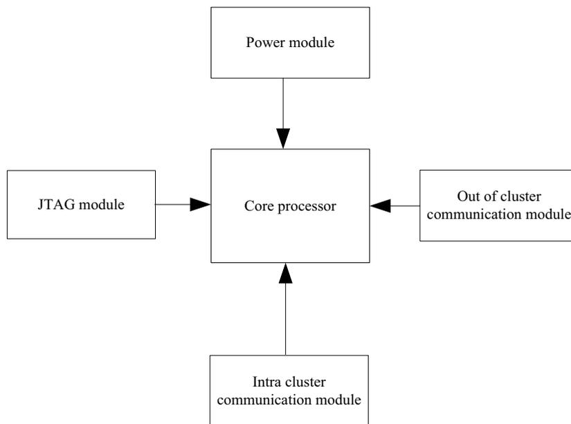
Fig. 4. Hardware structure diagram of distributed monitoring node module.
