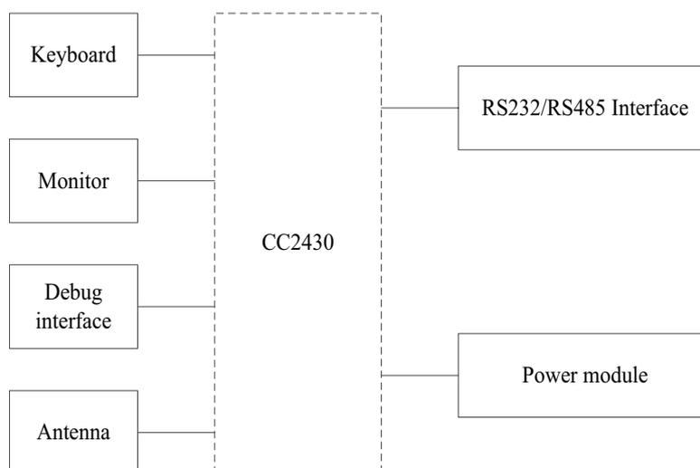
Fig. 2. Network coordinator structure diagram.
