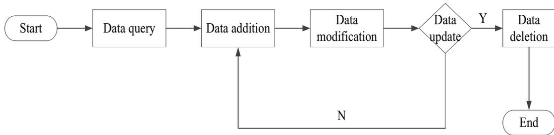
Fig. 3. Data management and maintenance module structure diagram.
