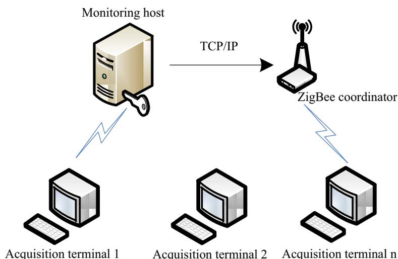
Fig. 1. The overall architecture design of the monitoring system.
