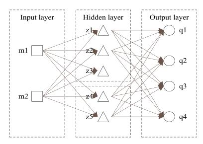
Fig. 6. Relationship between layers of BP neural network.
