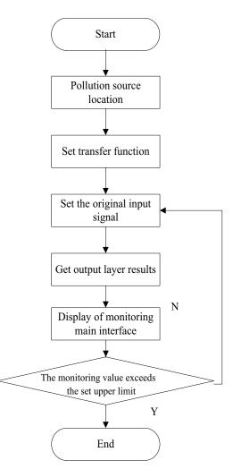
Fig. 7. Monitoring system software design process.
