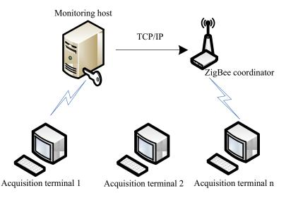
Fig. 1. The overall architecture design of the monitoring system.
