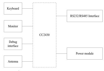
Fig. 2. Network coordinator structure diagram.
