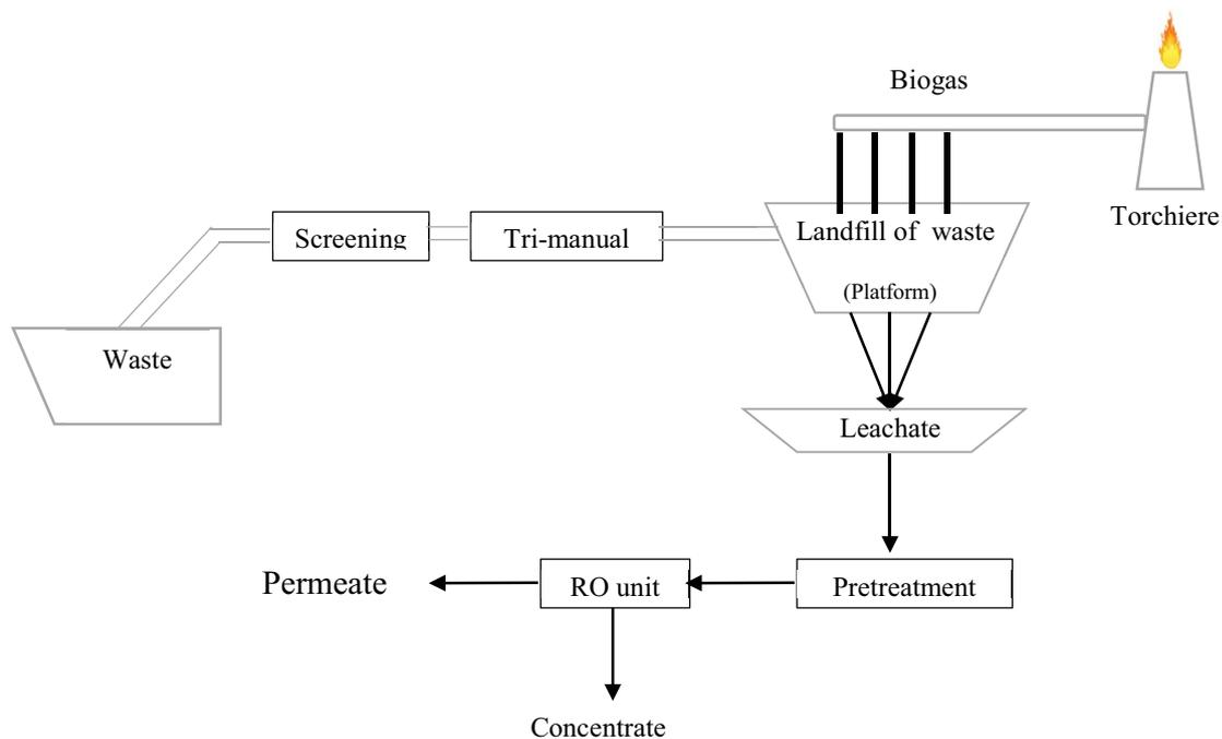
Fig. 1. Operating stages of the Oum Azza Landfill Plant.
