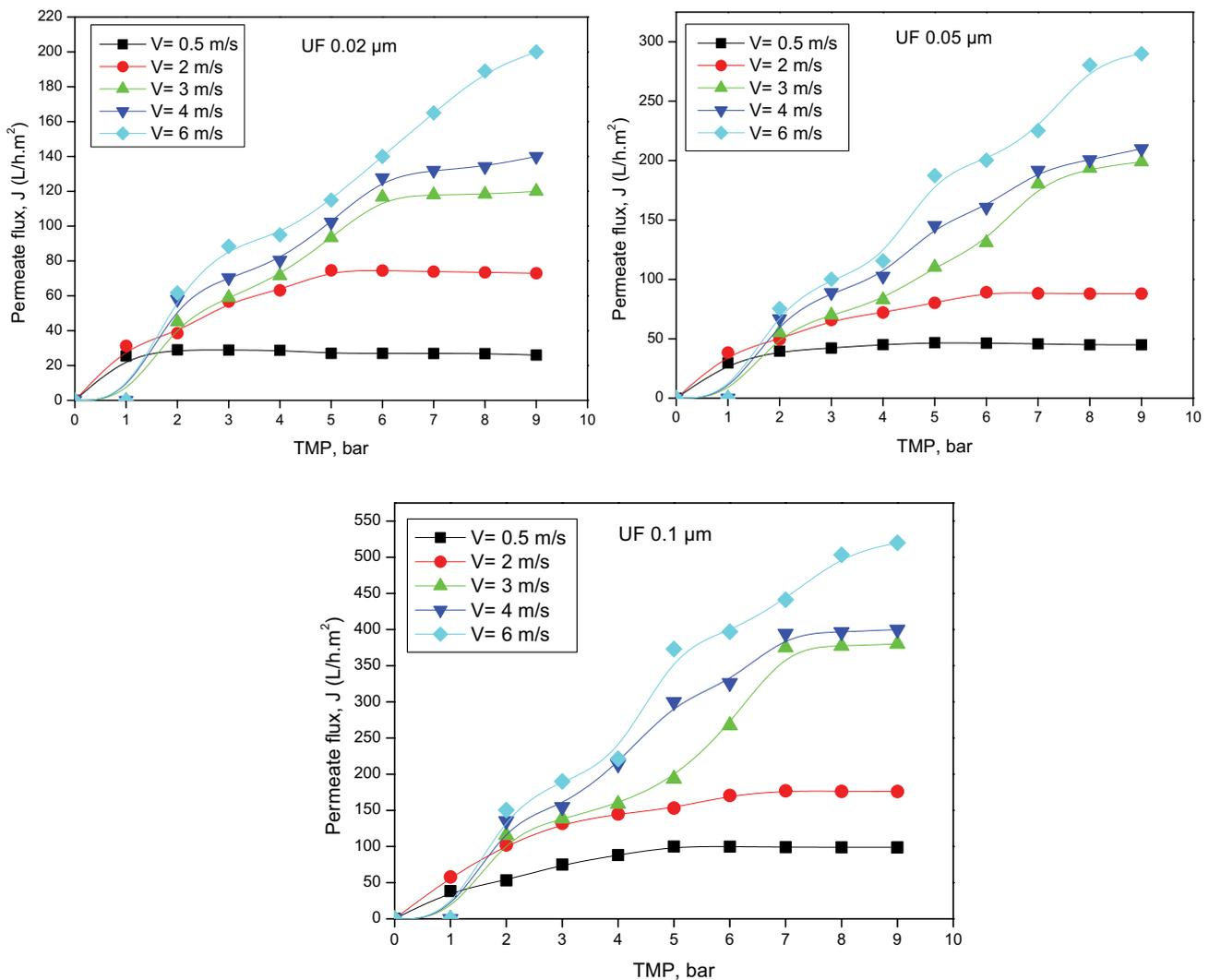
Fig. 6. Evolution of the permeation flux as a function of TMP at different circulation velocities for the three membranes studied (26°C).
