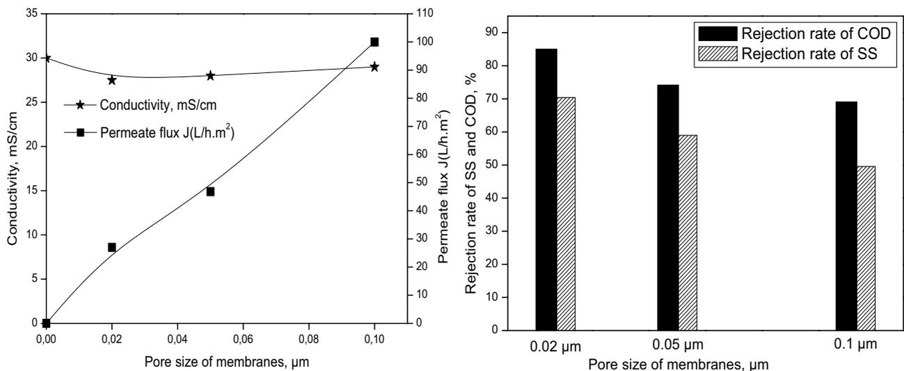
Fig. 4. Variation of flux, conductivity and retention of SS and COD as a function of pore size.
