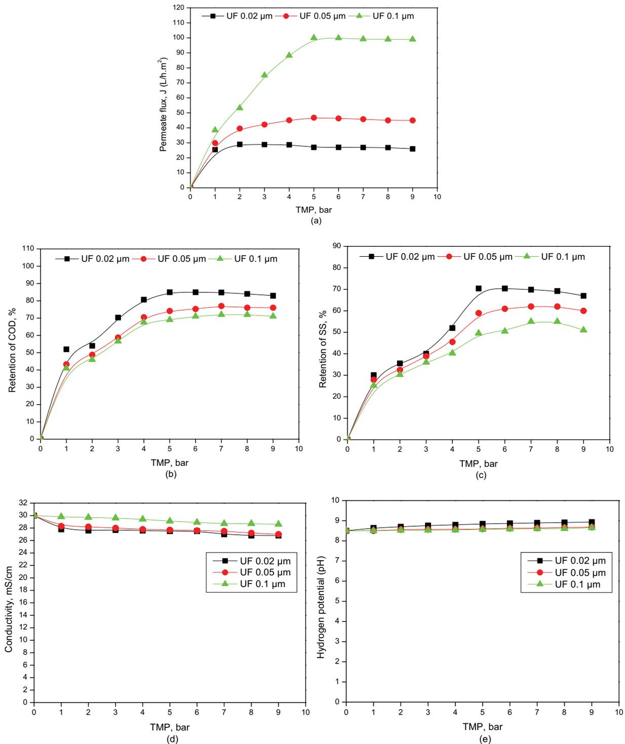
Fig. 5. Variations of permeate flux (a), COD (b) and SS (c) retention, electric conductivity (d) and pH (e) as a function of TMP ( $V = 0.5$  m/s).
