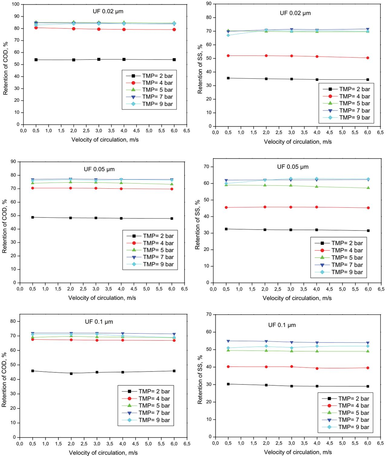
Fig. 7. Evolution of the COD and SS retentions as a function of circulation velocity for different TMP.
