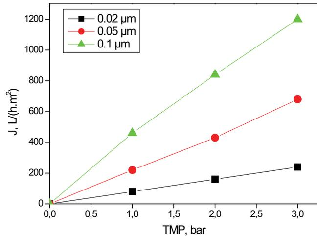
Fig. 3. The evolution of the water permeates flux as a function of TMP at 25°C.
