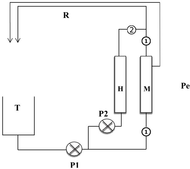
Fig. 2. Diagram of the ultrafiltration pilot plant. *T*: Tank; *P*<sub>1</sub>: Feed pump; *P*<sub>2</sub>: Filtration pump; *M*: Ultrafiltration module; *P*<sub>e</sub>: Permeate recirculation; *R*: Retentate recirculation; *H*: Heat exchanger; 1: Pressure sensor; 2: Temperature sensor.
