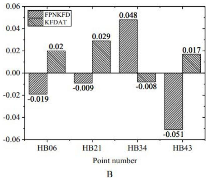
Fig. 5. The difference between kriging based on elevation abnormal terrain and fixed-point number kriging: (A) fitting value and (B) difference value.
