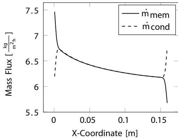
Fig. 6. Axial evaporation ( $\dot{m}_{\text{mem}}$ ) and condensation mass flux ( $\dot{m}_{\text{cond}}$ ) in mid  $z$  plane for 70°C hot inlet temperature.
