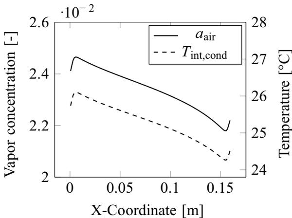
Fig. 7. Vapor concentration of air in the air-gap near the liquid film  $a_{air}$  and condensation interface temperature  $T_{int,cond}$  in mid  $z$  plane for 70°C hot inlet temperature; as  $T_{int,cond}$  is calculated from  $a_{air}$ , the curves are similar for small variations of  $T_{int,cond}$ .
