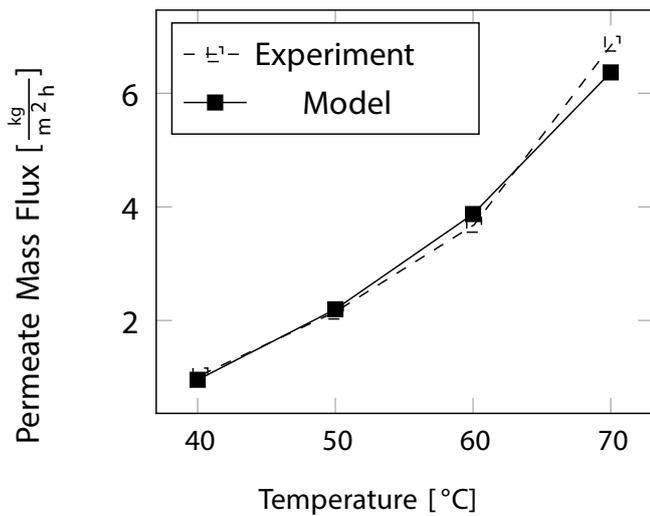
Fig. 4. Fresh water output for different hot salt water channel inlet temperatures; from the model the condensation mass flux  $\dot{m}_{\text{cond}}$  is used, the experiments are performed by Banat [32].
