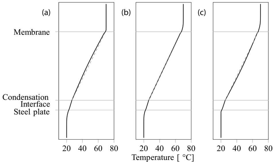
Fig. 5. The temperature profile in  $y$ -direction perpendicular to the membrane for 70°C hot inlet temperature (a) close to the hot water inlet ( $x = 0$  m), (b) in the mid- $X$  location ( $x = 0.8$  m) and (c) close to the hot water channel outlet and the coolant inlet ( $x = 0.16$  m); the dashed lines display a straight line between the temperatures at the membrane and at the condensation interface; deviations of the actual temperature profile (solid line) are due to natural convection.
