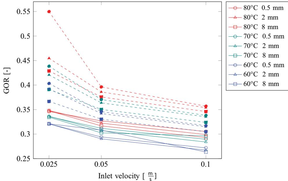
Fig. 11. GOR for different hot channel inlet temperatures, velocities and air-gap thicknesses:  $\circ$ —upside configuration;  $\bullet$ —downside configuration.
