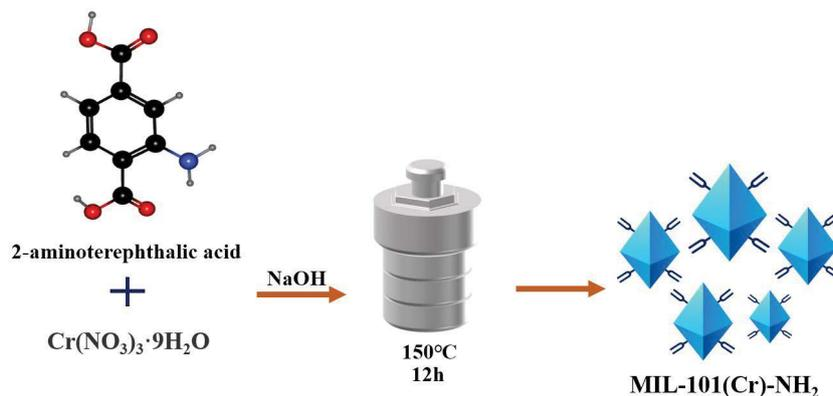
Fig. 1. Synthesis process of MIL-101(Cr)-NH<sub>2</sub>.
