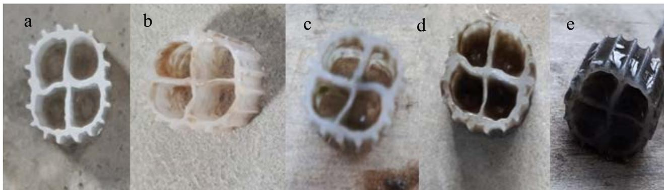
Fig. 2. Biofilm formation in the sequential oxic-anoxic bed reactor (SOABR). (a) day 1, (b) day 5, (c) day 10, (d) day 25, and (e) day 170.
