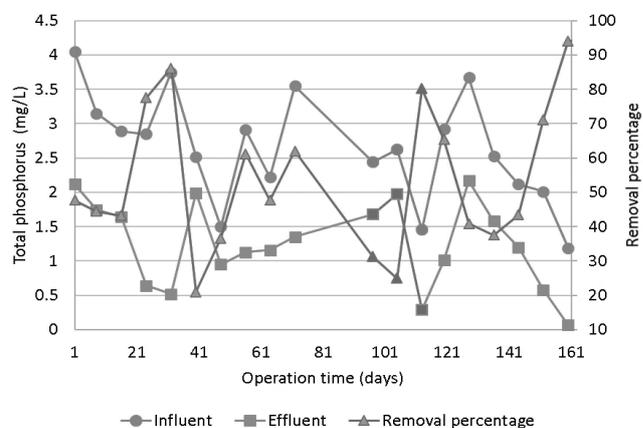
Fig. 8. Total phosphorus at the inlet and outlet of the fixed biomass.
