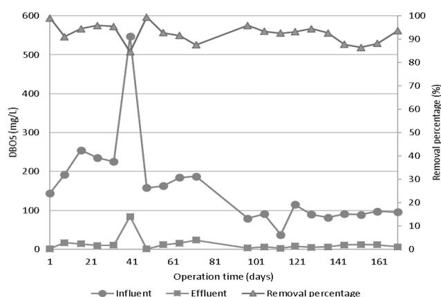
Fig. 5. BOD<sub>5</sub> at the inlet and outlet of the fixed biomass system.
