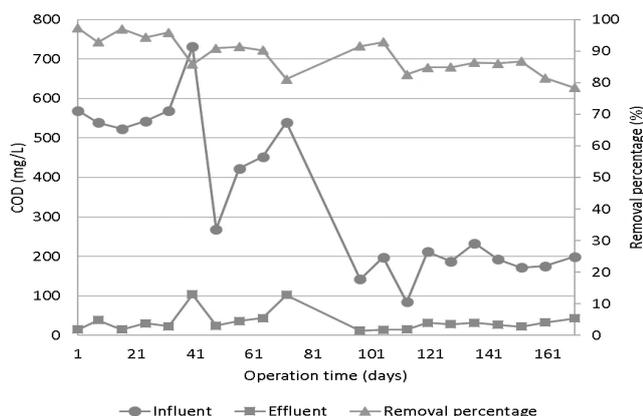
Fig. 6. Total COD in the inlet and outlet of the fixed biomass.
