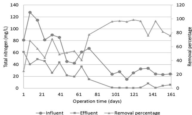
Fig. 7. Total nitrogen in the inlet and outlet of the fixed biomass.
