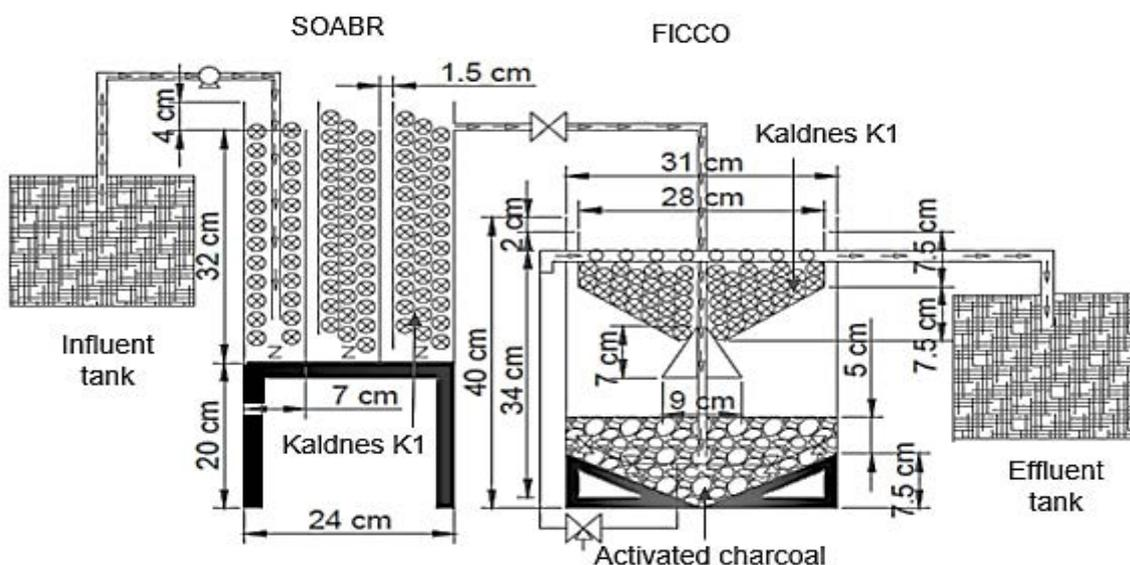
Fig. 1. Dimensions of the SOABR-FICCO system.
