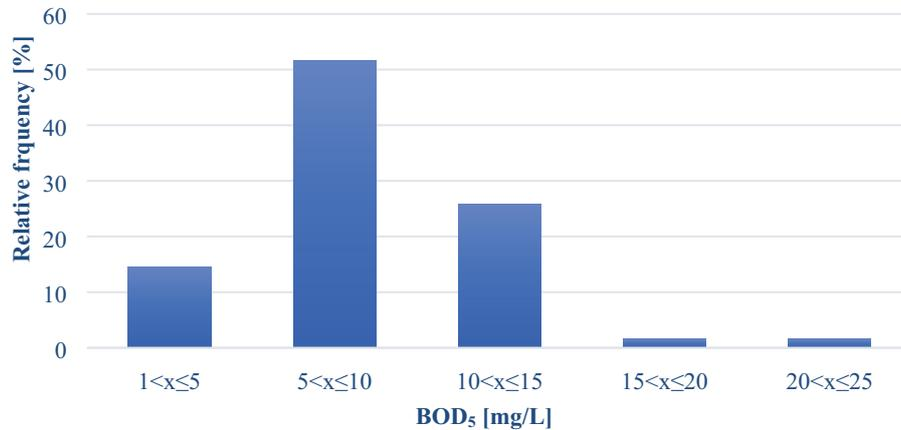
Fig. 9. Histogram of BOD<sub>5</sub> distribution in outflow.
