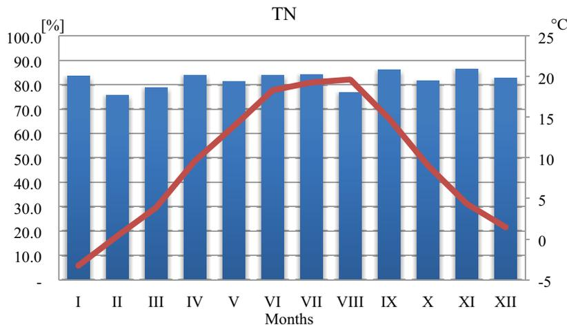
Fig. 14. Monthly average TN reduction efficiency and monthly average air temperature.
