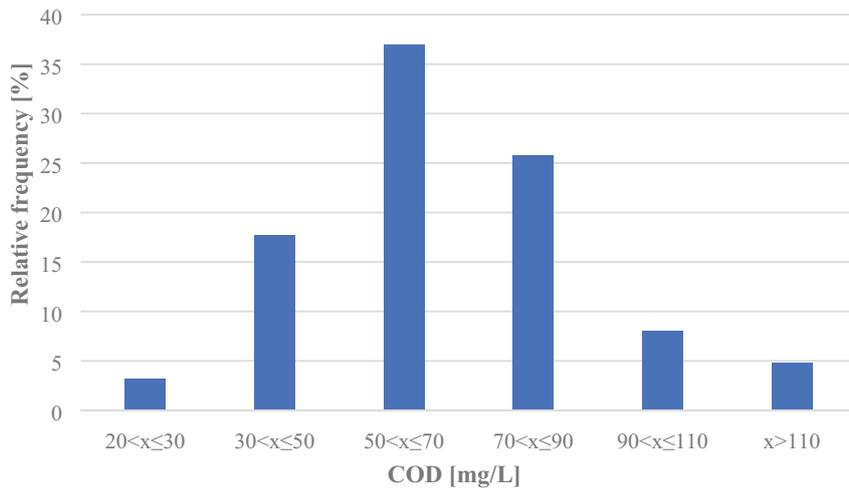
Fig. 11. Histogram of COD distribution in outflow.
