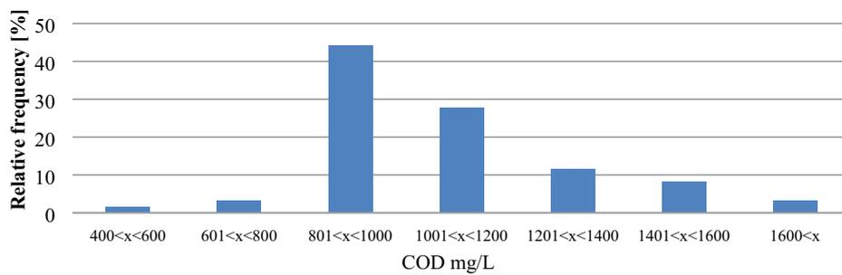
Fig. 3. Histogram of COD distribution in raw sewage.
