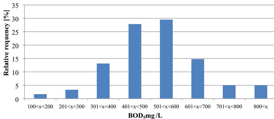
Fig. 5. Histogram of BOD<sub>5</sub> distribution in raw sewage.
