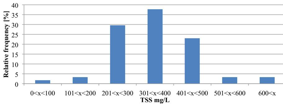
Fig. 4. Histogram of TSS distribution in raw sewage.
