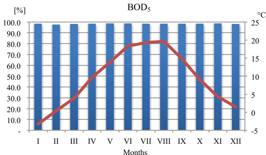
Fig. 8. Average monthly BOD<sub>5</sub> reduction efficiency and monthly average air temperature.
