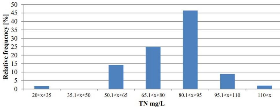
Fig. 6. Histogram of TN distribution in raw sewage.
