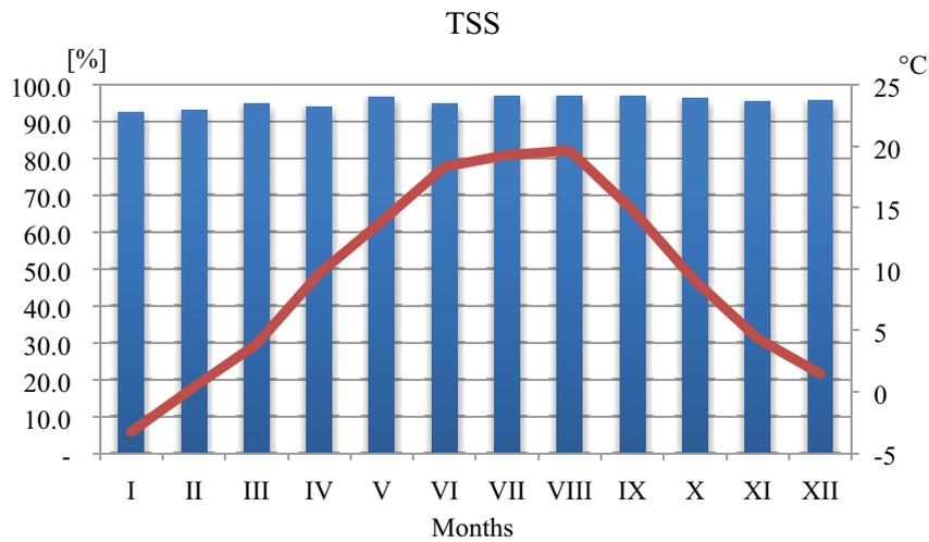
Fig. 12. Average monthly TSS reduction efficiency and monthly average air temperature.
