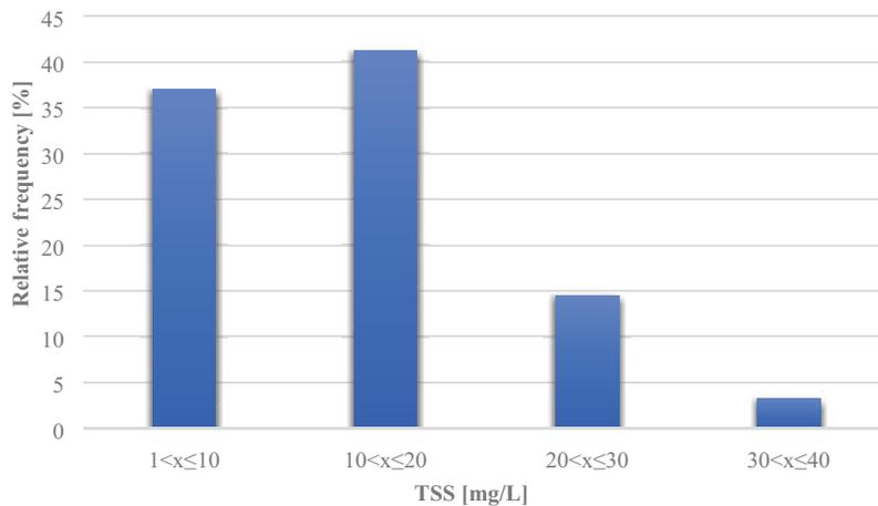
Fig. 13. Histogram of TSS distribution in outflow.
