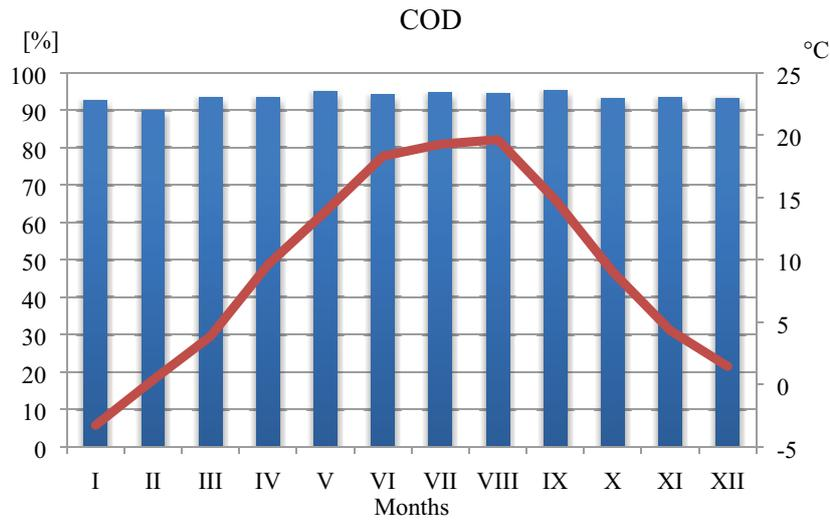
Fig. 10. Average monthly COD reduction efficiency and monthly average air temperature.
