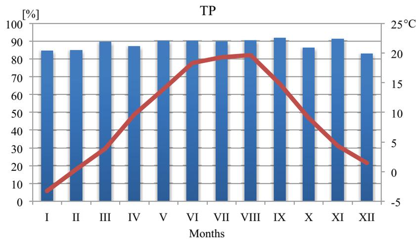
Fig. 16. Average monthly TP reduction efficiency and monthly average air temperature.
