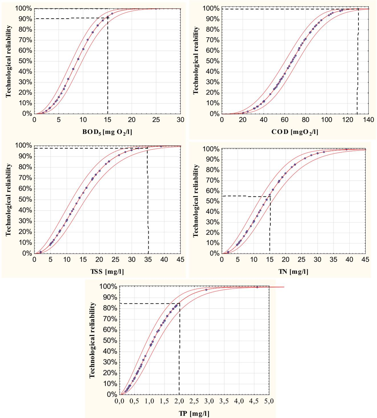
Fig. 18. Weibull cumulative distribution functions and the technological reliabilities determined for each pollution parameter. Notation: dashed red line – reliability function; dashed black line – probability of achieving the indicators limit in the effluent (Regulation 2019).
