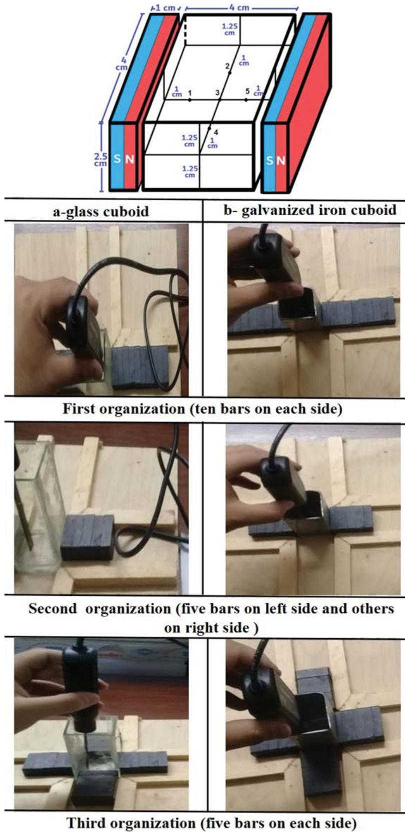
Fig. 8. Measurement locations of the magnetic intensity of horizontal magnetic field (first case: cuboid with square base: 4 cm × 4 cm).
