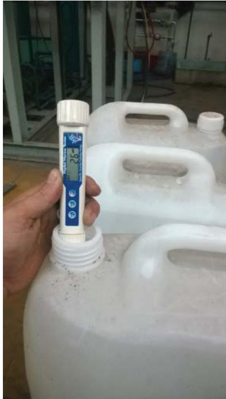
Fig. A3. Checking the salinity of seawater.
