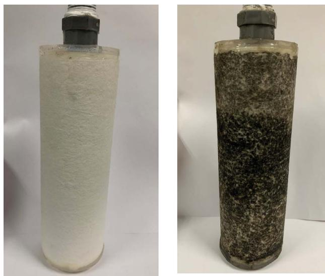
Fig. 1. Photographs of PP fiber filter membrane (left) and GO-PP fiber filter membrane (right).
