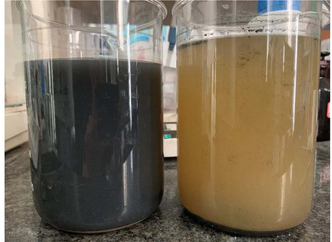
Fig. 4. Comparison of water-based paint waste before (left) and after (right) flocculation.
