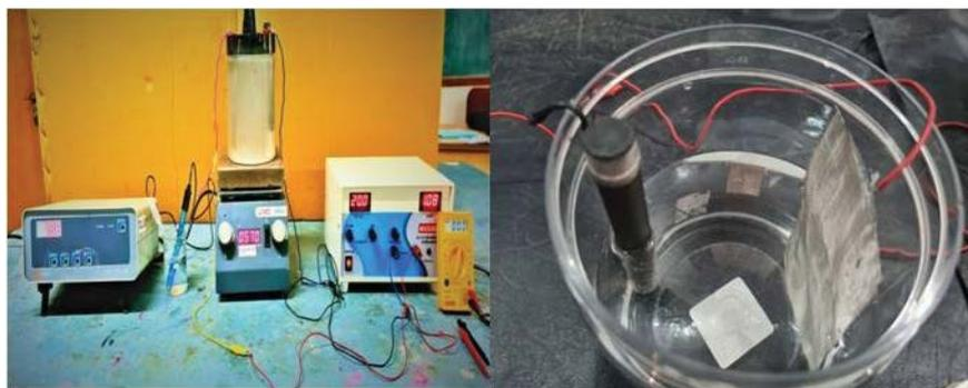
Fig. 2. Photograph of the electrochemical setup.
