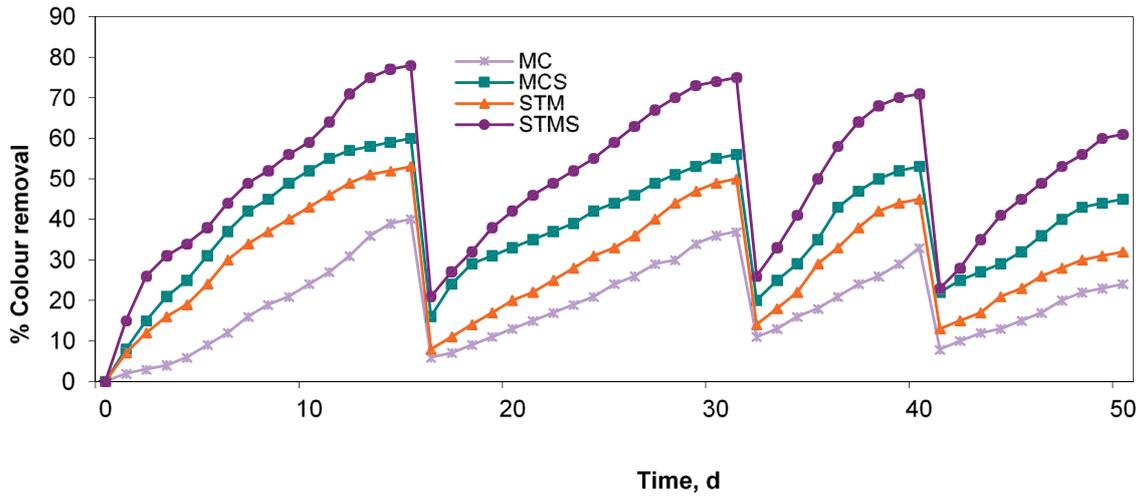
Fig. 7. Colour removal during tannery wastewater treatment in SBR – 6,240 mg COD/L.
