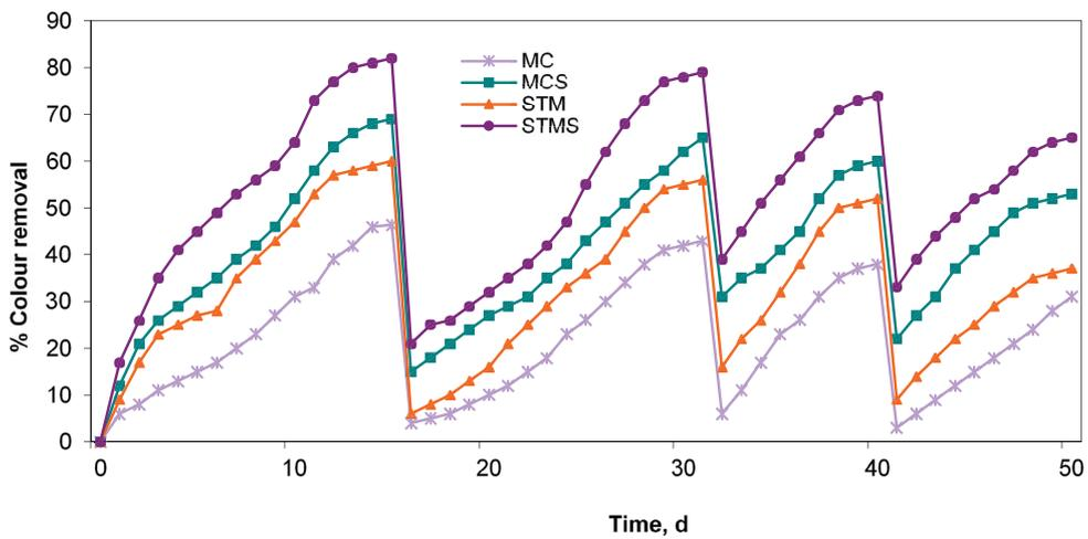
Fig. 6. Colour removal during tannery wastewater treatment in SBR – 4,680 mg COD/L.
