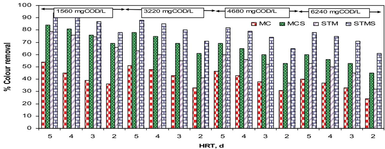
Fig. 9. Effect of HRT on colour removal efficiency.
