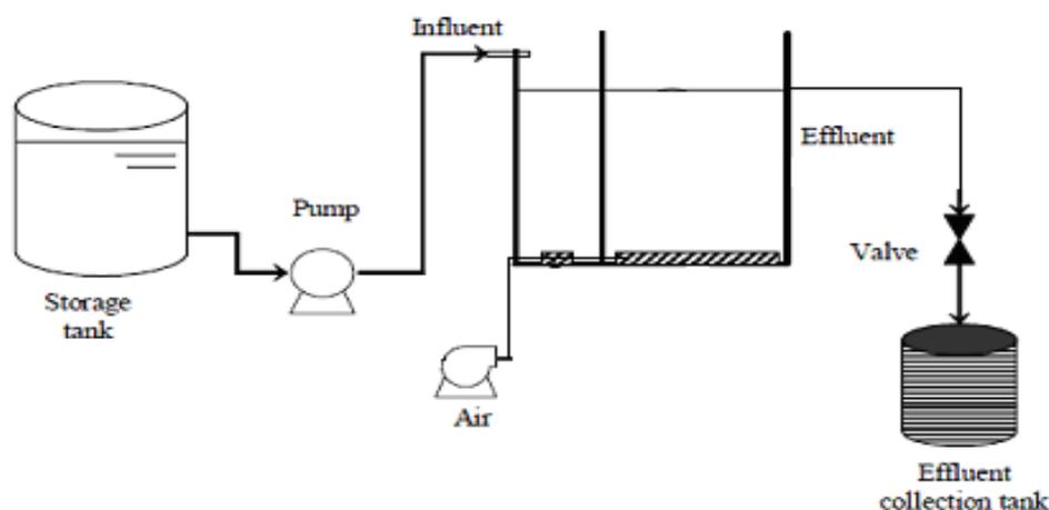
Fig. 1. Schematic of sequential batch reactor set up.
