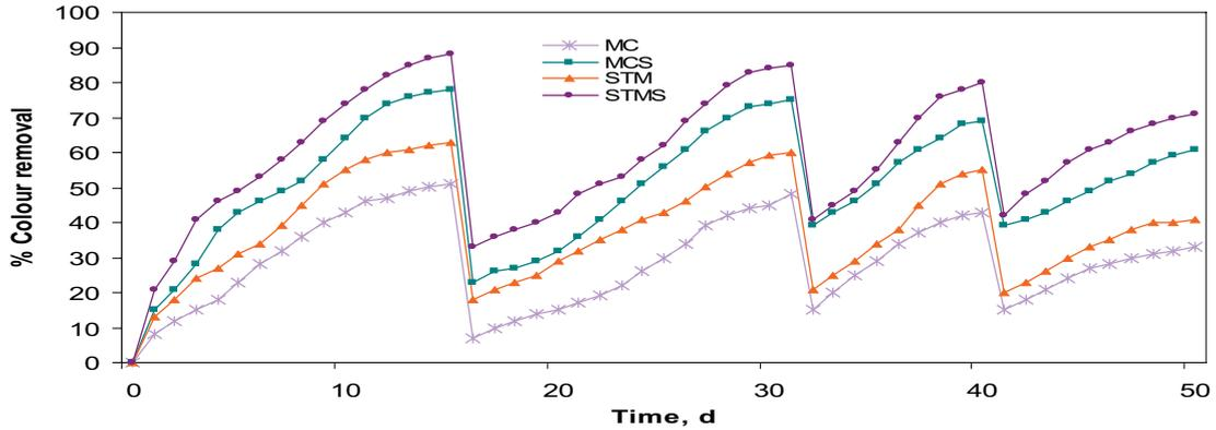
Fig. 5. Colour removal during tannery wastewater treatment in SBR – 3,220 mg COD/L.
