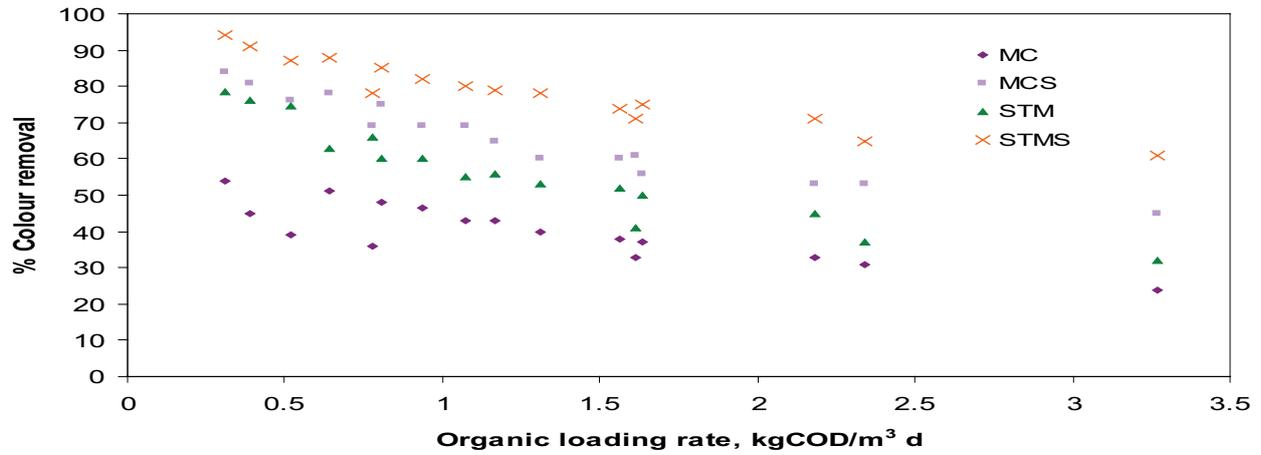
Fig. 8. Effect of organic loading rate on colour removal efficiency.
