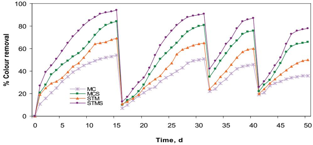
Fig. 4. Colour removal during tannery wastewater treatment in SBR – 1,560 mg COD/L.
