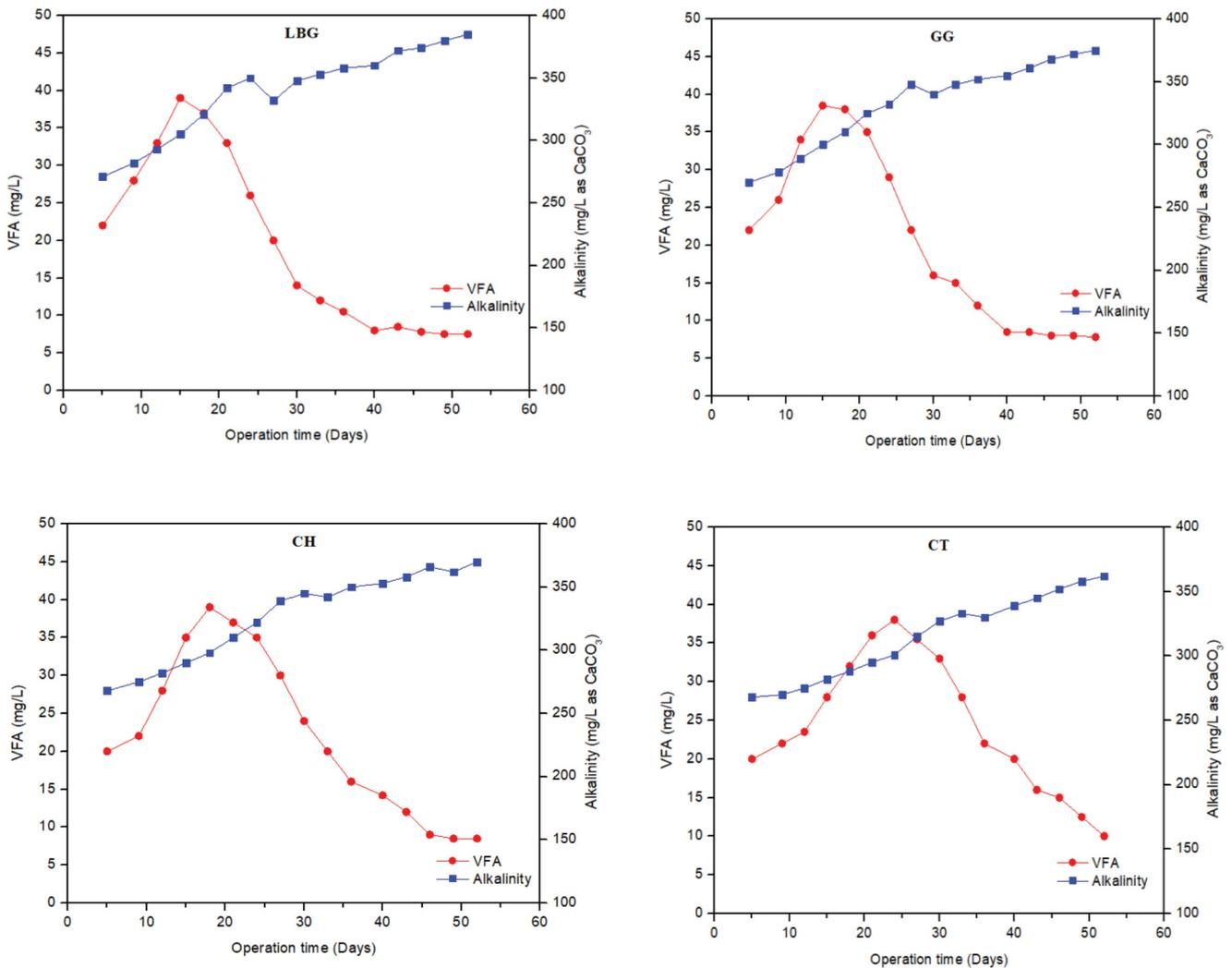
Fig. 5. Interplay of alkalinity and VFA for LBG, GG, CH and CT reactors – startup phase.
