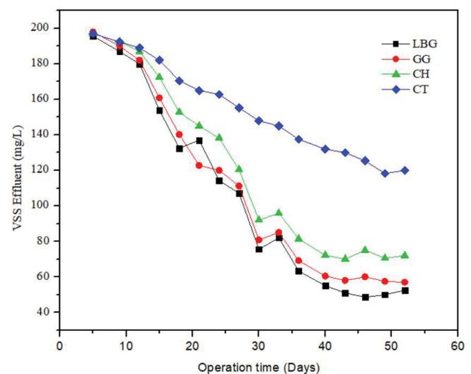
Fig. 3. Comparison of VSS concentration in the effluent.
