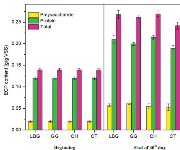
Fig. 8. Variation of ECP content in the sludge at the beginning and end of startup phase.
