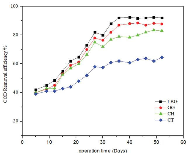
Fig. 2. COD removal efficiency for the startup phase.
