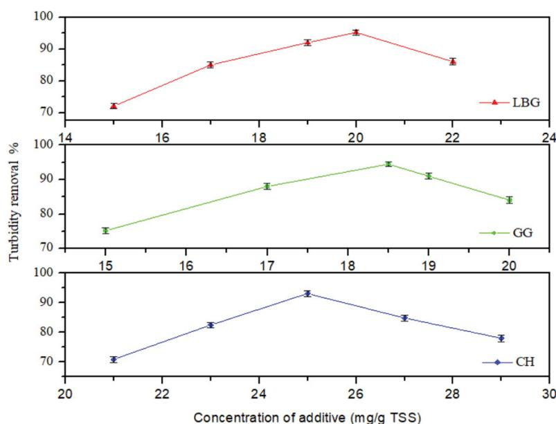
Fig. 1. Turbidity removal efficiencies of the chosen additives at varied concentrations.
