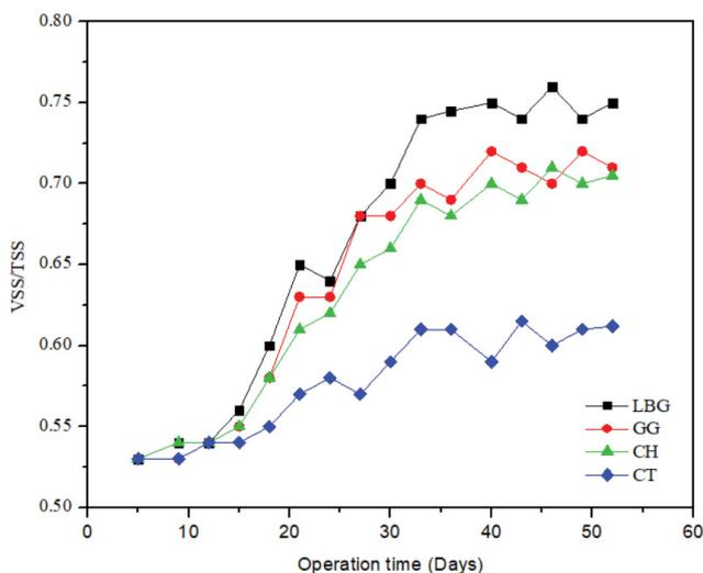
Fig. 6. Comparative study of VSS/TSS ratio of granules from different reactors.
