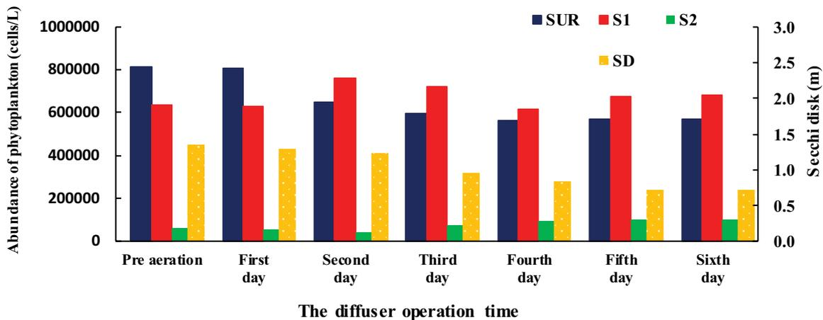
Fig. 8. Vertical distribution of algae at different sampling stations and Secchi disk transparency during the aeration.
