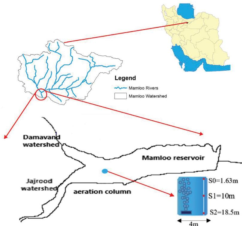
Fig. 1. The map of the study area: The watershed and Mamloo Reservoir, and the schematic aeration column with the monitoring stations.
