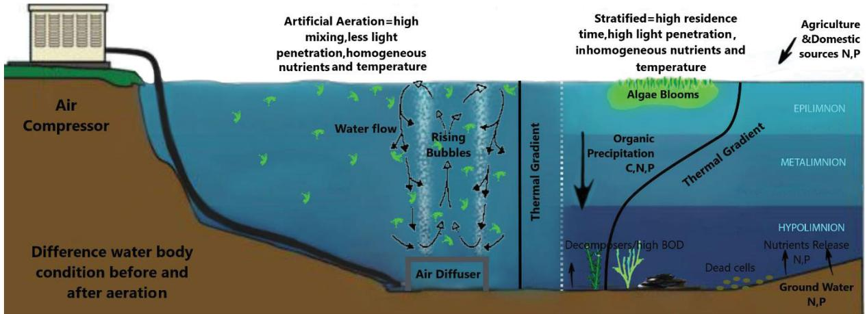
Fig. 2. Schematic diagram of artificial mixing and stratified condition in reservoir.
