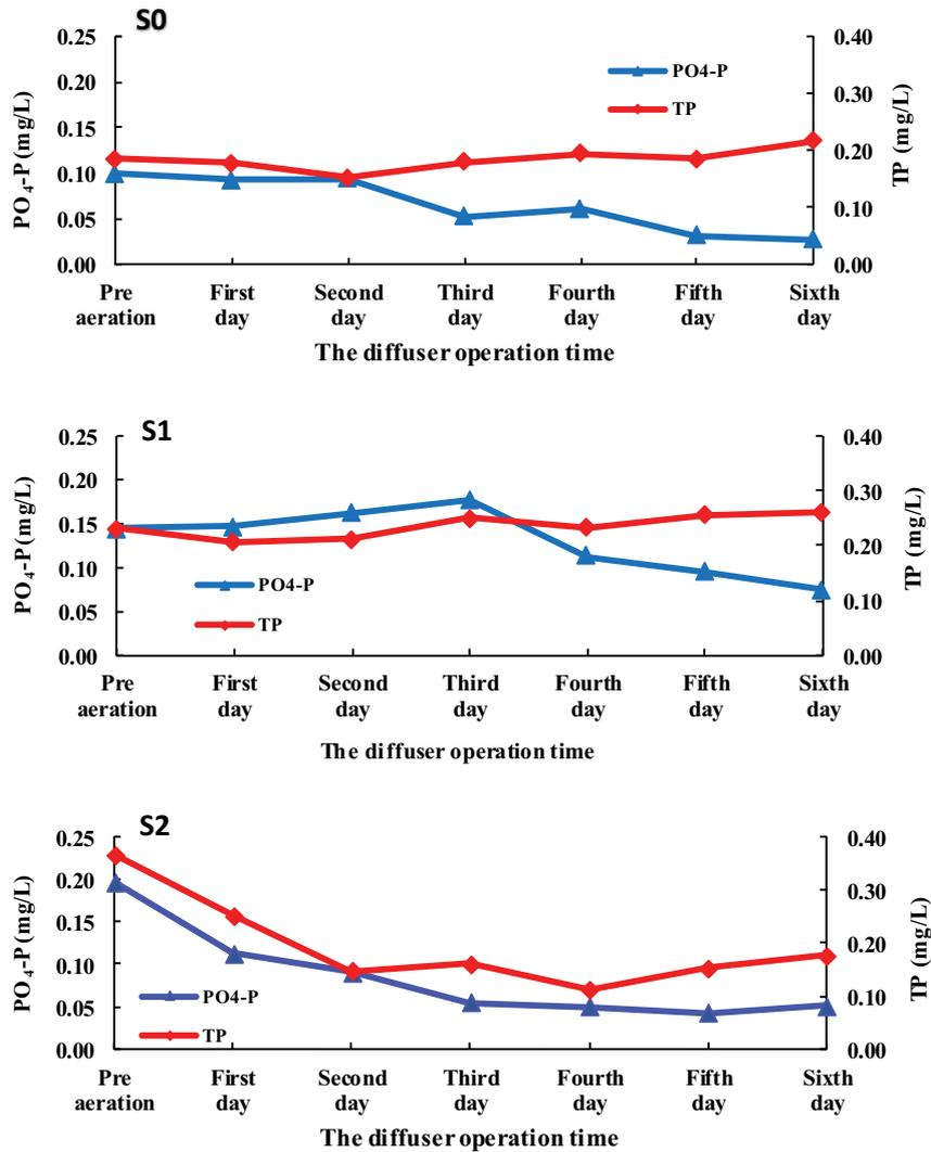
Fig. 6. Dynamic change of soluble reactive phosphorus (PO<sub>4</sub>-P) and total phosphorus (TP), during the aeration in S0–S2.
