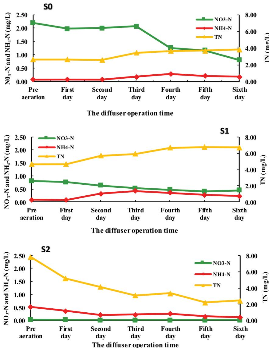
Fig. 5. Dynamic change of ammonium (NH<sub>4</sub>-N), nitrate (NO<sub>3</sub>-N) and total nitrogen (TN) during the aeration in S0–S2.
