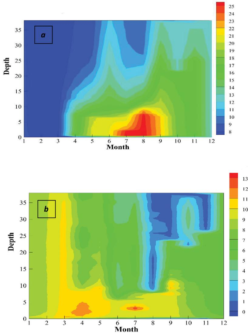
Fig. 3. Vertical variation of (a) water temperature (°C) and (b) dissolved oxygen (mg/L) in MLOR at the different months of 2019, at the depth of 37 m.
