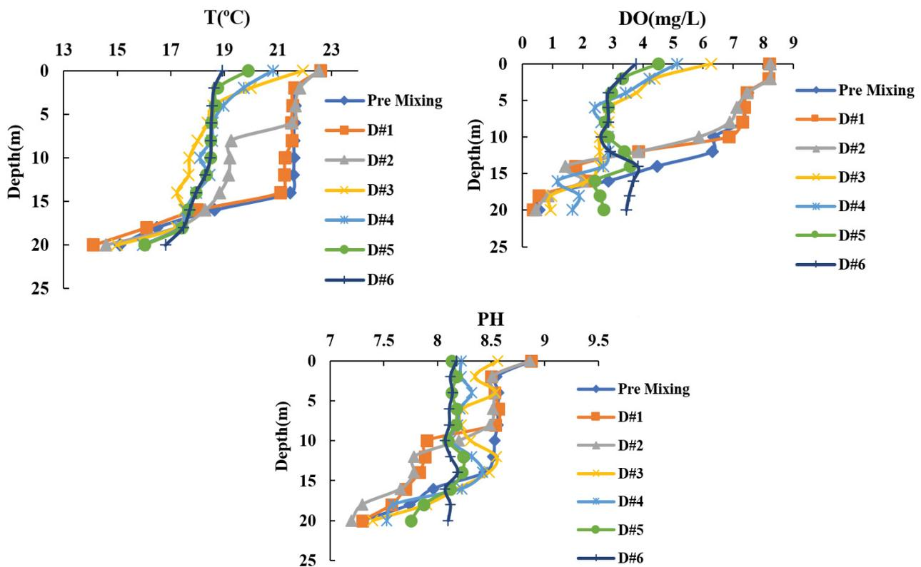
Fig. 4. Daily vertical variation of water temperature, DO, and pH value, during the aeration.
