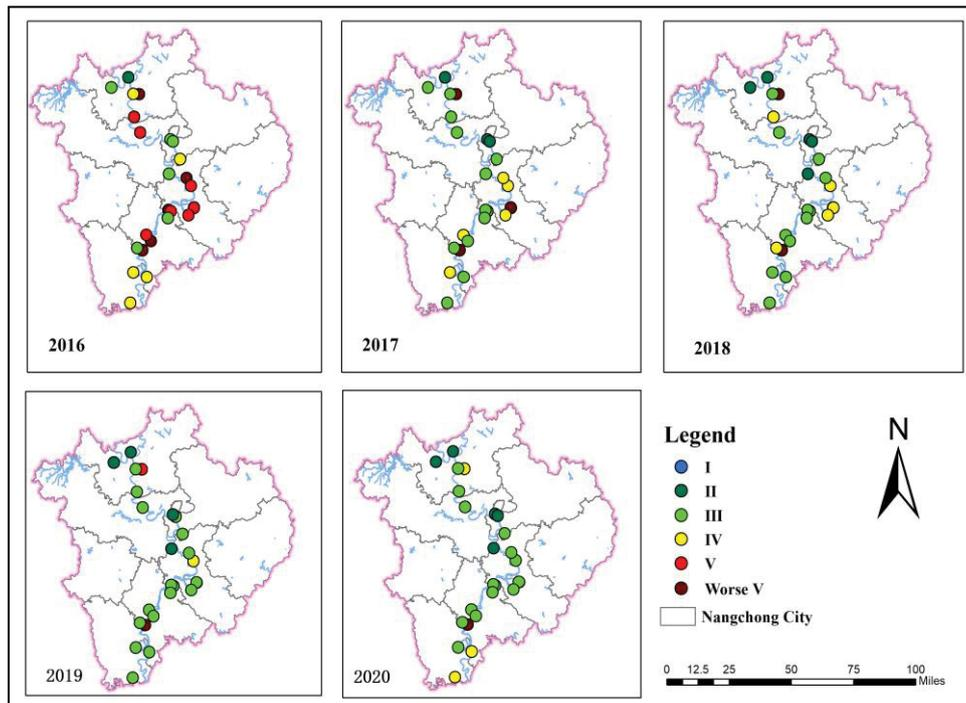
Fig. 3. Spatial GIS distribution of single-factor evaluation results of the first-level tributaries in Nanchong Section of Jialing River.
