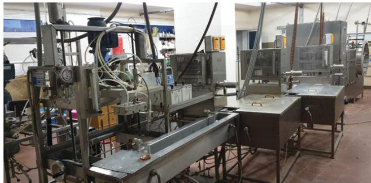
Fig. 2. Photo of adopted pilot-scale spinning system.
