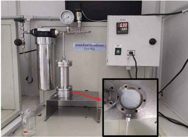
Fig. 4. Dead-end test (pure water permeation set-up).
