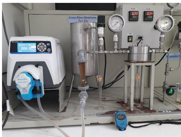
Fig. 3. CFR test configuration (filtration set).
