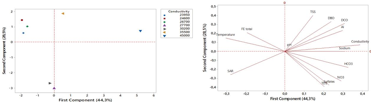
Fig. 18. Principal component analysis (PCA) of wastewater physico-chemical parameters.
