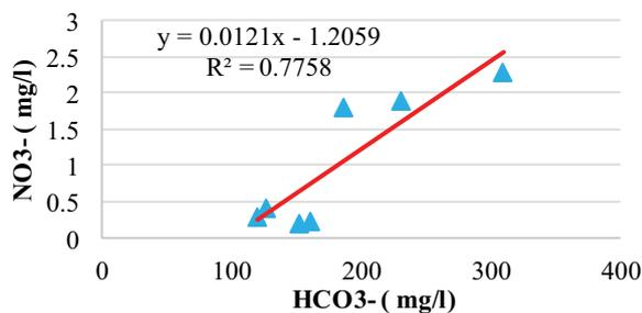
Fig. 15. Linear plot between NO<sub>3</sub><sup>-</sup> and HCO<sub>3</sub><sup>-</sup>.
