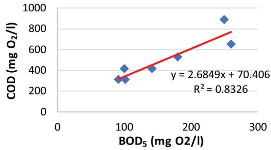
Fig. 13. Linear plot between COD and BOD<sub>5</sub>.
