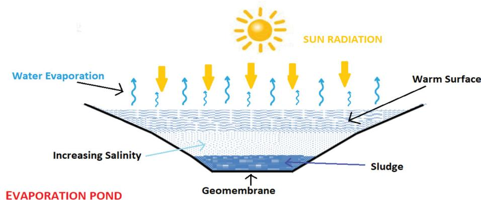
Fig. 1. Evaporation pond illustration.
