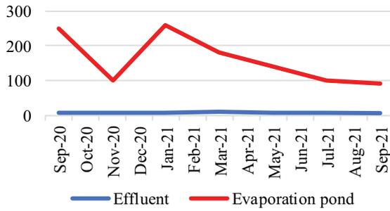
Fig. A4. BOD<sub>5</sub> (mg O<sub>2</sub>/L) analysis results.
