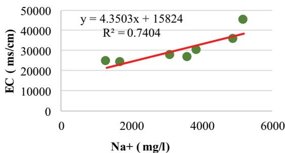
Fig. 8. Linear plot between EC and Na<sup>+</sup>.
