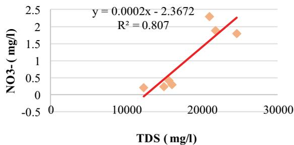
Fig. 16. Linear plot between NO<sub>3</sub><sup>-</sup> and TDS.
