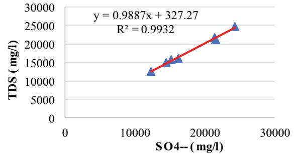
Fig. 17. Linear plot between TDS and SO<sub>4</sub><sup>-</sup>.
