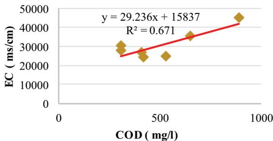
Fig. 7. Linear plot between EC and COD.
