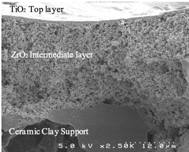
Fig. 7. Scanning electron micrographs of TiO<sub>2</sub> membrane.
