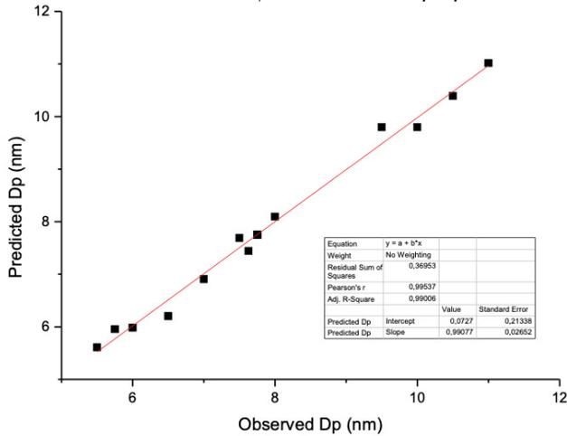
Fig. 2. Parity plot of predicted vs. observed responses for pore diameter ( $D_p$ ).
