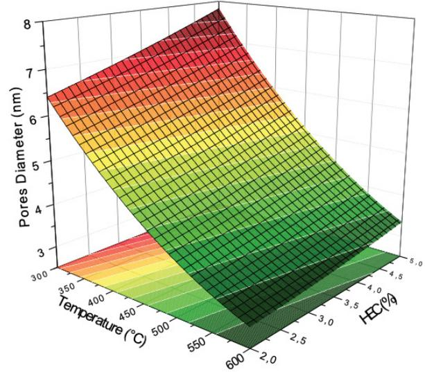
Fig. 6. Response surface plot of pores diameter of ultrafiltration membrane vs. temperature and HEC.
