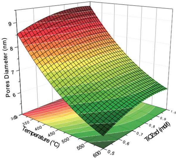
Fig. 5. Response surface plot of pores diameter of ultrafiltration membrane vs. temperature and TiO<sub>2</sub> sol.
