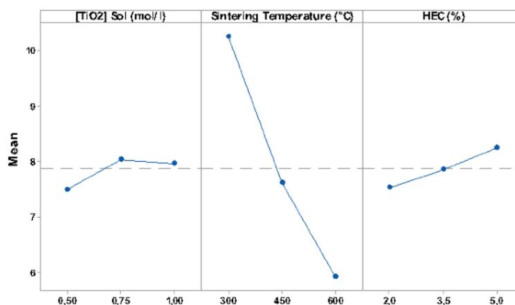
Fig. 4. Main effects for pore diameter.
