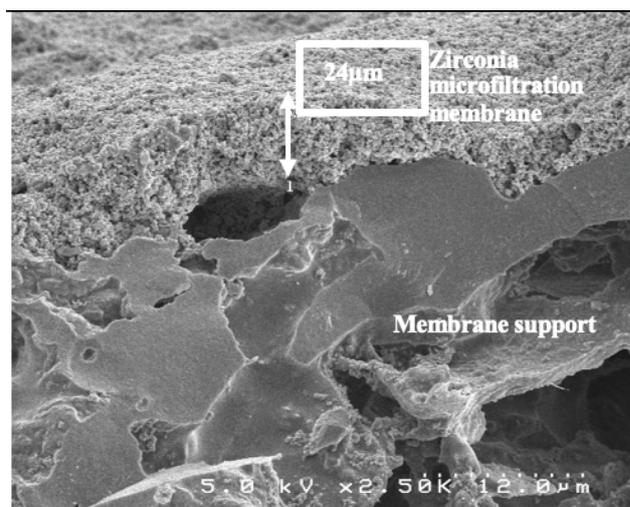
Fig. 1. Scanning electron micrographs of membrane support and zirconia microfiltration layer.
