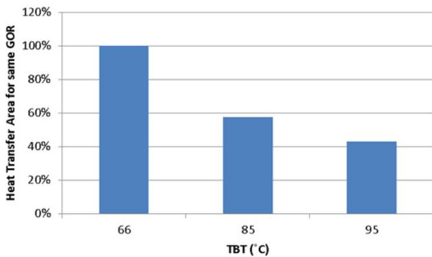
Fig. 7. Decrease in heat transfer area with increase of TBT with the same GOR.
