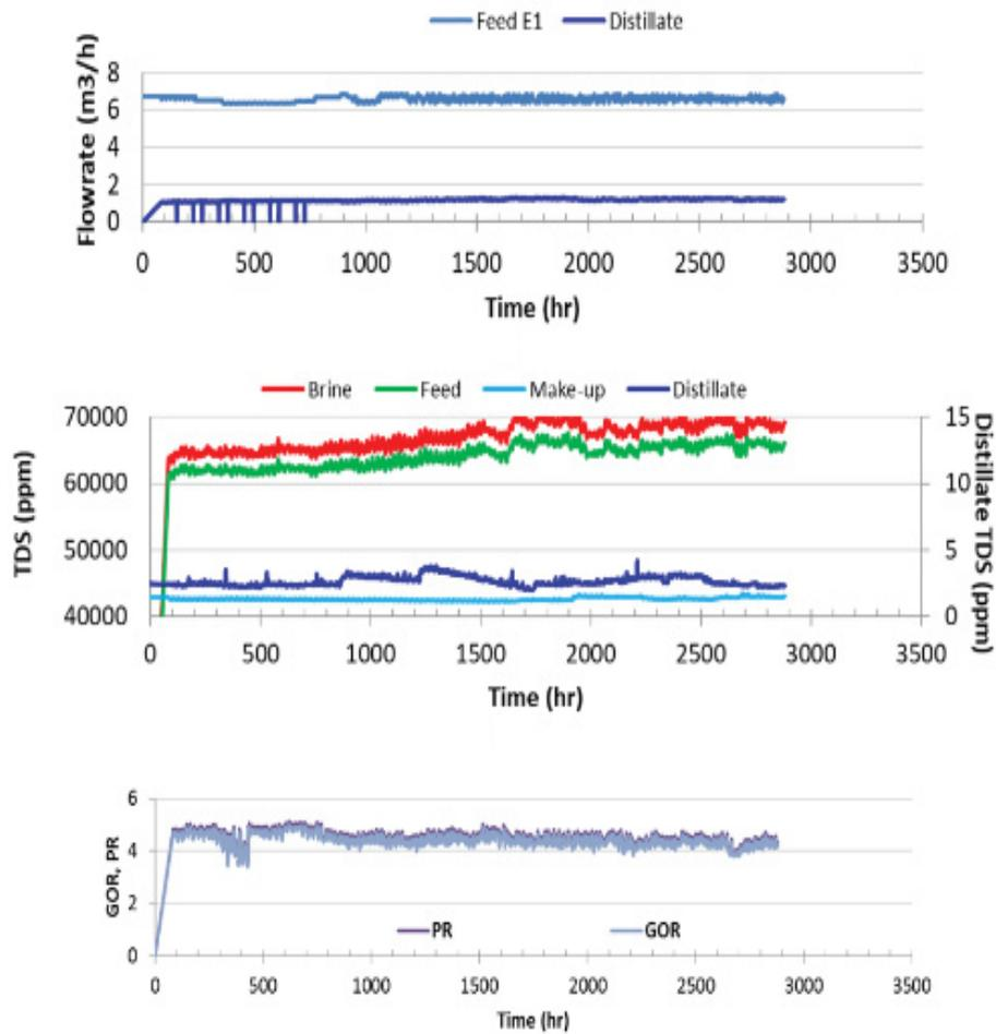
Fig. 5. Profiles of flow rates, concentrations, PR and GOR. Distillate TDS is shown on the secondary y-axis.
