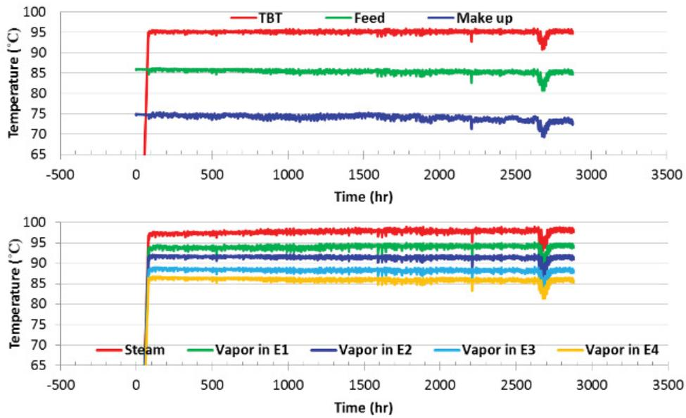
Fig. 4. Temperature profiles of top brine temperature, feed, make-up seawater temperature, steam and vapor temperature in individual effect.
