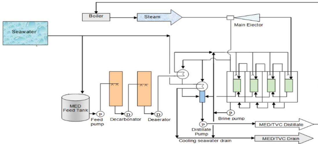
Fig. 2. The flow diagram of MED-TVC process.
