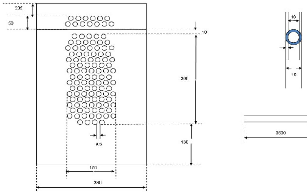
Fig. 3. Two pass arrangement of the tube bundles. Also shown are the diameter, the thickness and the length of the tubes.
