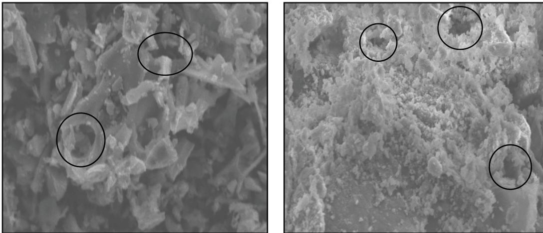
Fig. 2. Surface physical morphology of WGMS (a) before and (b) after adsorption.
