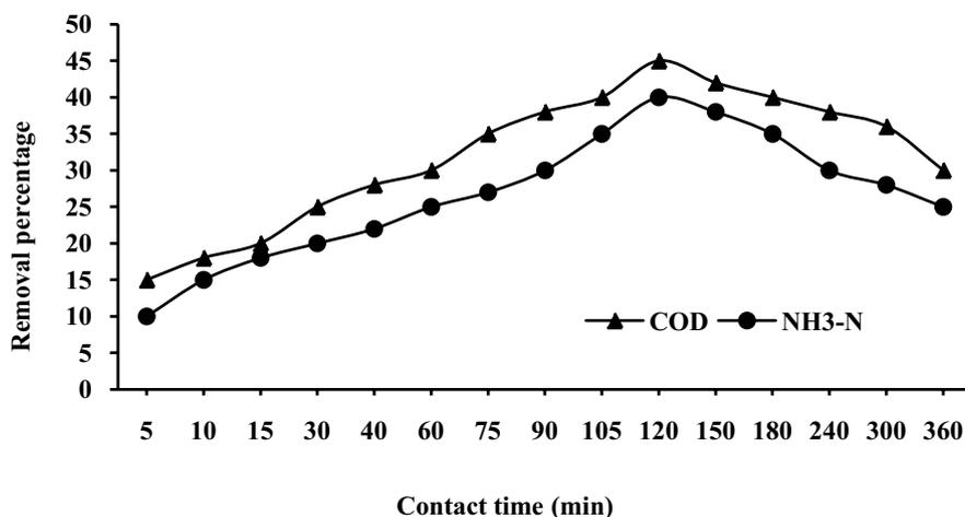
Fig. 5. Percentage of COD and  $\text{NH}_3\text{-N}$  removal against different contact time.
