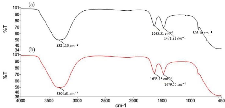
Fig. 1. FTIR spectra of waste green mussel shell (a) before and (b) after treatment.
