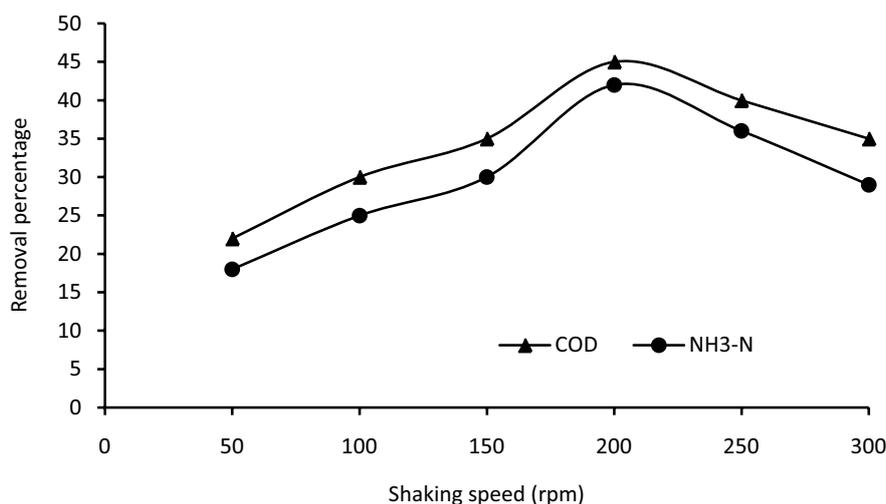
Fig. 4. Percentage of COD and  $\text{NH}_3\text{-N}$  removal against different shaking speed.
