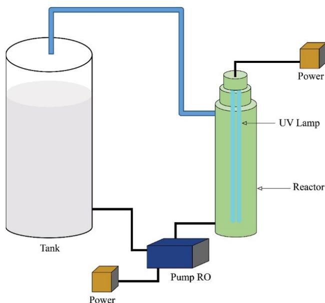
Fig. 1. Schematics of the test setup.
