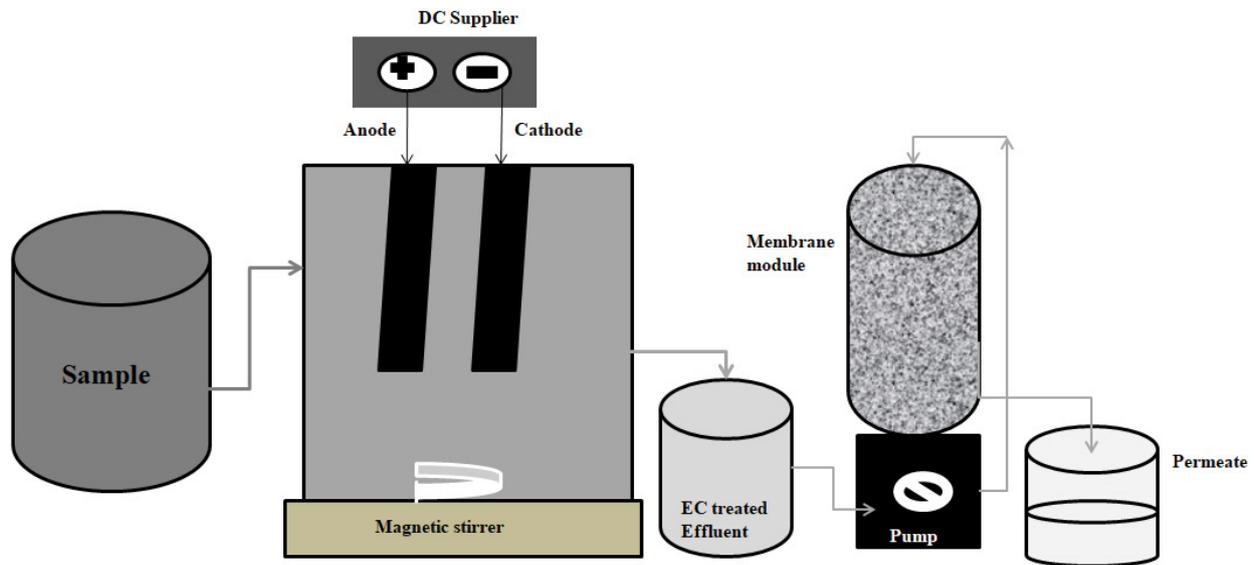
Fig. 1. Schematic diagram of the EC-MF bench scale units
