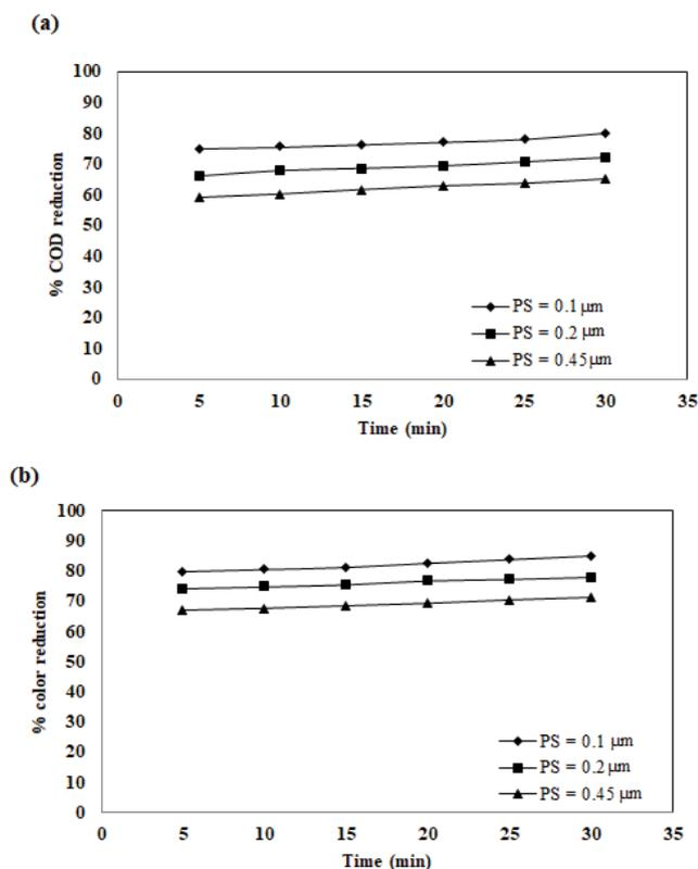
Fig. 10. Effect of PS on (a) percentage COD reduction and (b) color reduction (feed = untreated effluent, COD concentration = 7,020 mg/dm<sup>3</sup>, color = 485 PCU, feed flow rate = 1.1 L/min, feed pressure = 20 kPa).
