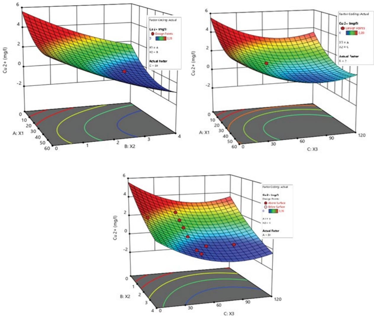
Fig. 8. 3D response surfaces of the effect of the interaction between the three parameters (time ( $X_1$ ), mass of resin ( $X_2$ ), stirring speed ( $X_3$ )) of concentration [ $\text{Cu}^{2+}$ ].
