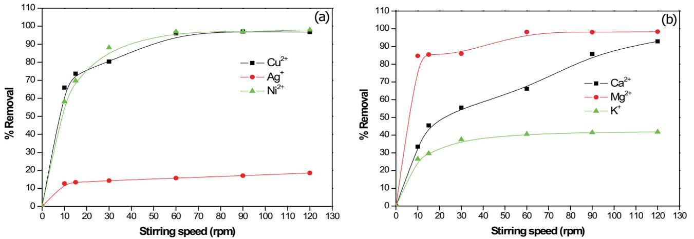
Fig. 6. Removal of Cu<sup>2+</sup>, Ag<sup>+</sup>, Ni<sup>2+</sup> (a) and Ca<sup>2+</sup>, Mg<sup>2+</sup>, K<sup>+</sup> (b) by Lewatit S 1568 resin vs. stirring speed.
