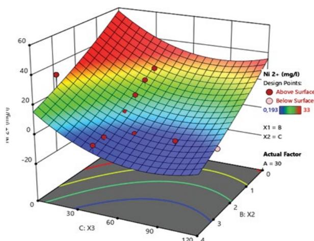
Fig. 10. 3D response surfaces of the effect of the interaction between the three parameters (time ( $X_1$ ), mass of resin ( $X_2$ ), stirring speed ( $X_3$ )) of concentration [ $\text{Ni}^{2+}$ ].
