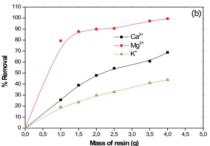
Fig. 4. Removal of  $Cu^{2+}$ ,  $Ag^+$ ,  $Ni^{2+}$  (a) and  $Ca^{2+}$ ,  $Mg^{2+}$ ,  $K^+$  (b) vs. mass of resin.
