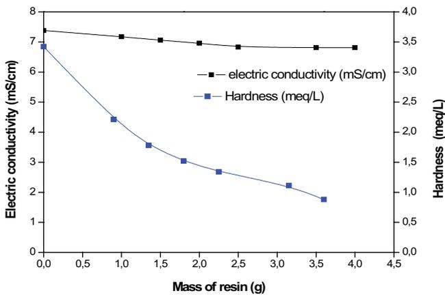
Fig. 3. Electric conductivity and hardness vs. mass of resin.
