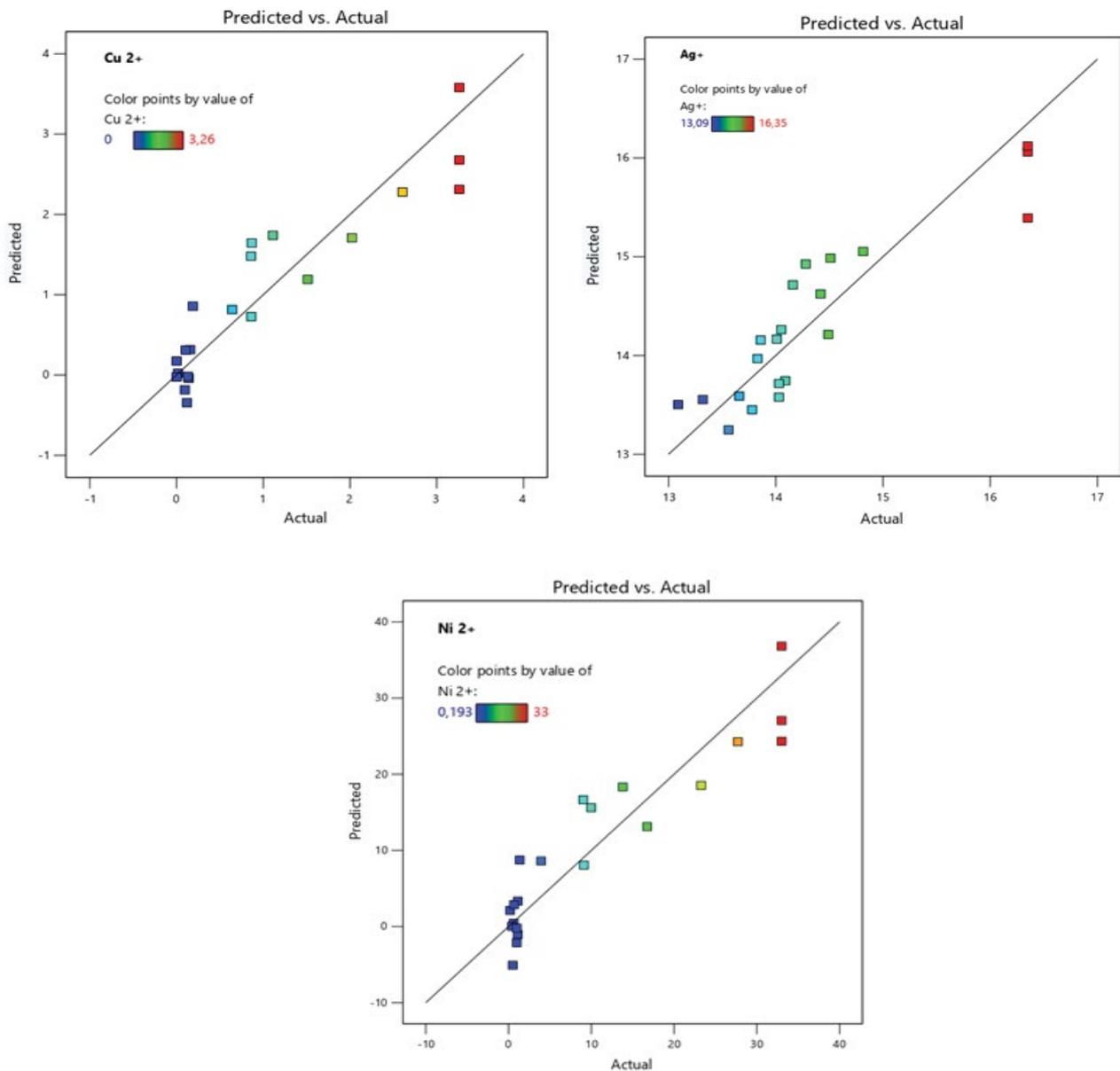
Fig. 7. Experimental data vs. predicted data of the responses ( $[Cu^{2+}]$ ,  $[Ag^+]$  and  $[Ni^{2+}]$ ) calculated by applying the regression Eqs. (2)–(4).
