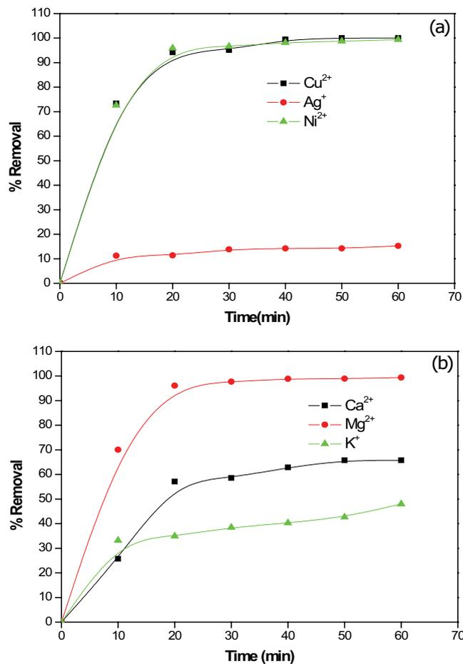
Fig. 2. Effect of contact duration on removal of  $\text{Cu}^{2+}$ ,  $\text{Ag}^+$ ,  $\text{Ni}^{2+}$  (a) and  $\text{Ca}^{2+}$ ,  $\text{Mg}^{2+}$ ,  $\text{K}^+$  (b) by IER.
