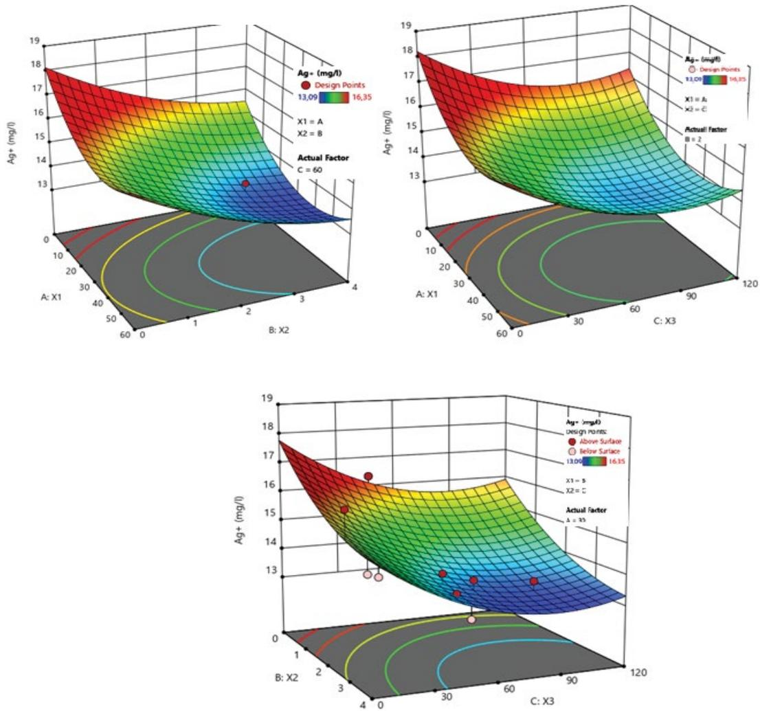
Fig. 9. 3D response surfaces of the effect of the interaction between the three parameters (time ( $X_1$ ), mass of resin ( $X_2$ ), stirring speed ( $X_3$ )) of concentration [ $Ag^+$ ].
