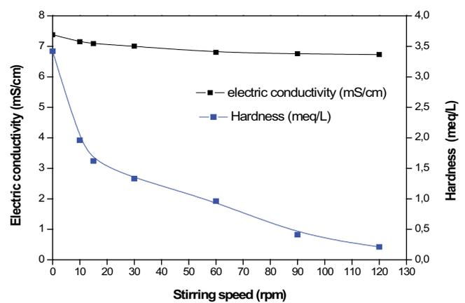
Fig. 5. Electric conductivity and hardness vs. stirring speed.
