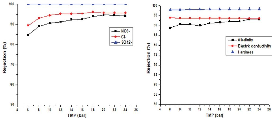
Fig. 4. Rejection of nitrate, chloride, sulfate, electric conductivity alkalinity and hardness vs. TMP.
