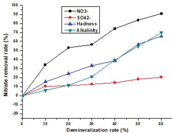
Fig. 3. Variation of the electric conductivity of the dilute and nitrate removal rate, alkalinity and sulfate as a function of demineralization rate (DR).
