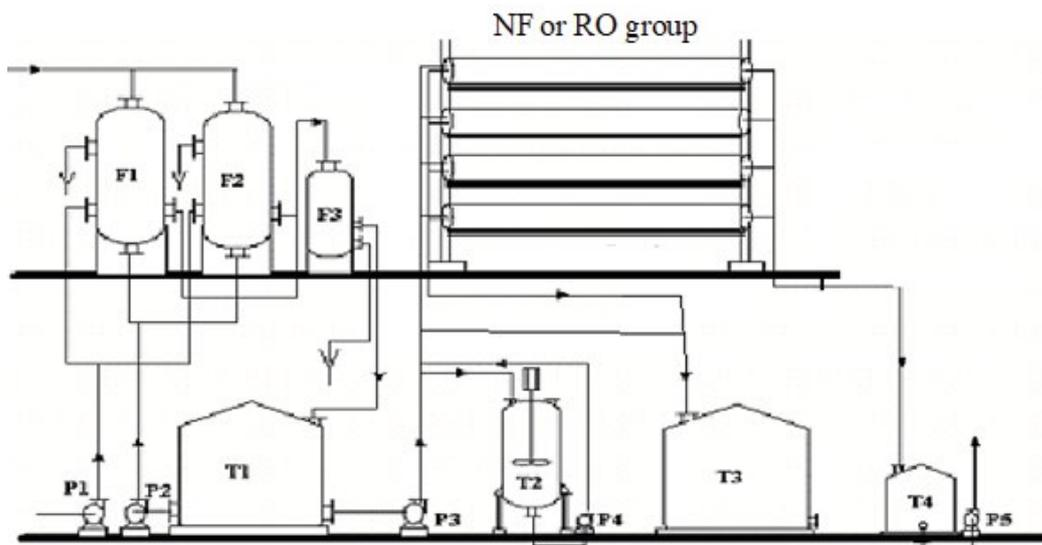
Fig. 10. Design of NF and RO plant for nitrate removal. F1 and F2 Sand filters, F3 Cartridge filter, T2 Sequestering preparation tank, T3 Treated water tank, T4 Brine tank.
