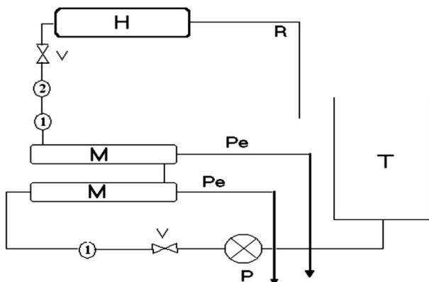
Fig. 2. Schematic diagram of RO/NF pilot plant. P: Feed pump; V: Pressure regulation valves; M: Reverse osmosis/nanofiltration module; Pe: Permeate recirculation; R: Retentate recirculation; H: Heat exchanger; 1: Pressure sensor; 2: Temperature sensor.
