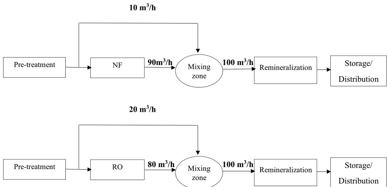
Fig. 8. Proposed design for nitrate removal by NF and RO.
