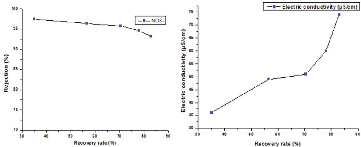
Fig. 7. Nitrate rejection and electric conductivity vs. recovery rate.
