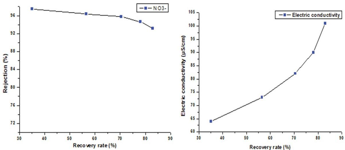
Fig. 5. Rejection of nitrate and electric conductivity as function of recovery rate.
