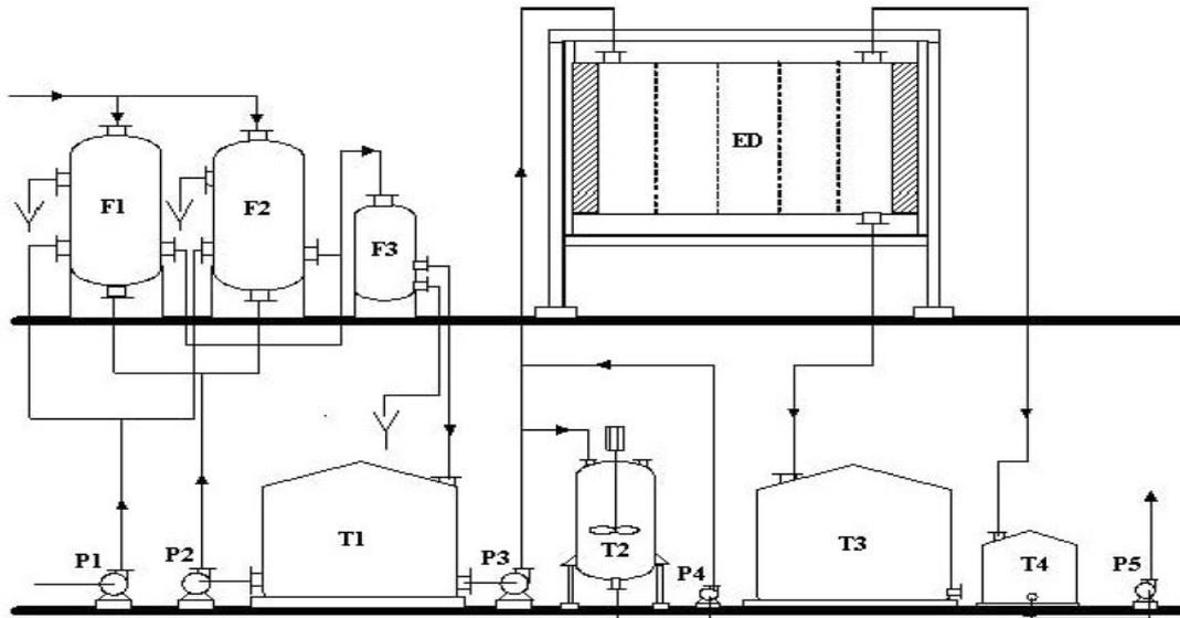
Fig. 9. Scheme of ED plant for nitrate removal. F1 and F2 Sand filters, F3 Cartridge filter, T2 Sequestering preparation tank, T3 Treated water tank, T4 Brine tank.
