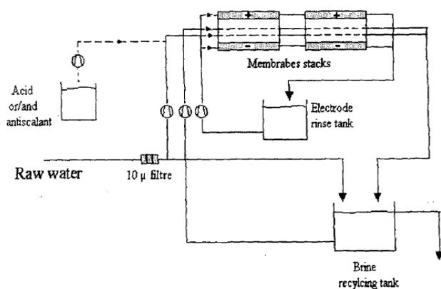
Fig. 1. Schematic diagram of ED pilot plant.
