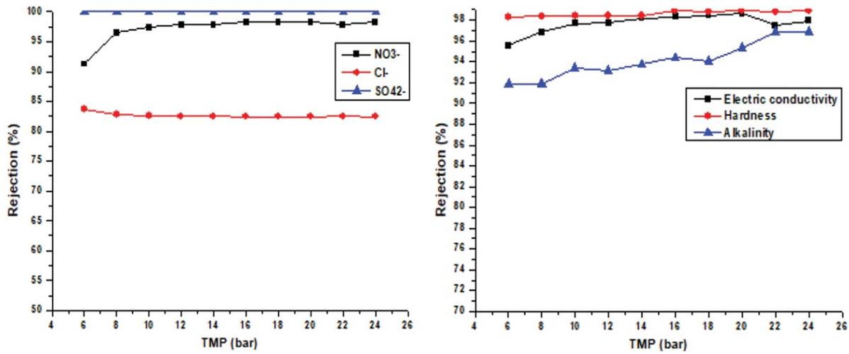
Fig. 6. Rejection of nitrate, chloride, sulfate, electric conductivity, alkalinity and hardness as function of TMP.
