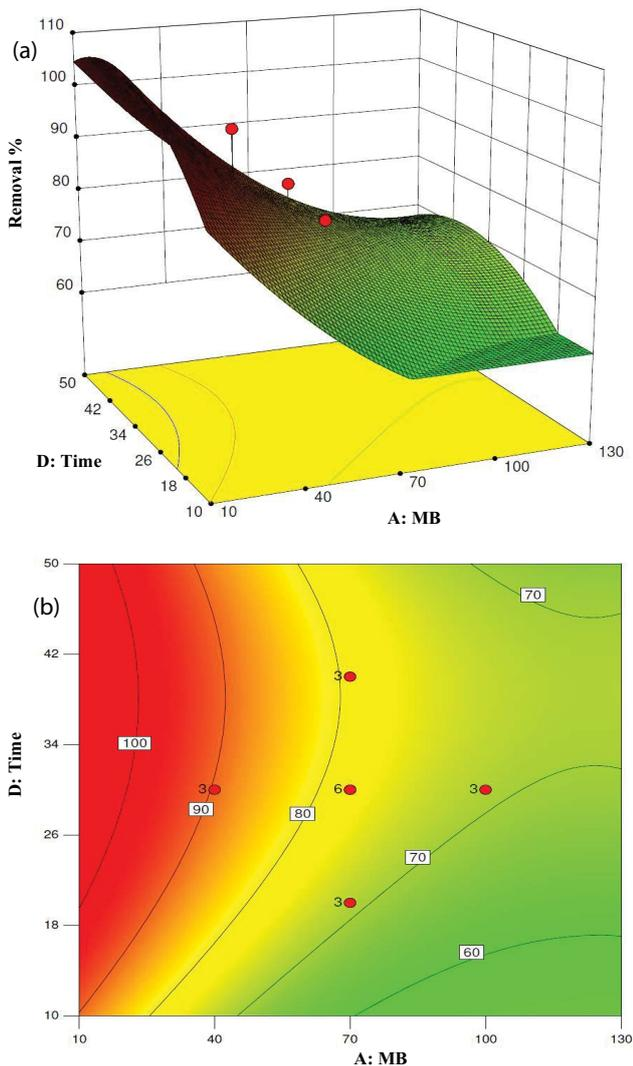
Fig. 6. Response surface plots (a) and response contour plot (b) of MB concentration and contact time in the removal of MB (pH = 7 and AC dosage = 0.8 g/L).
