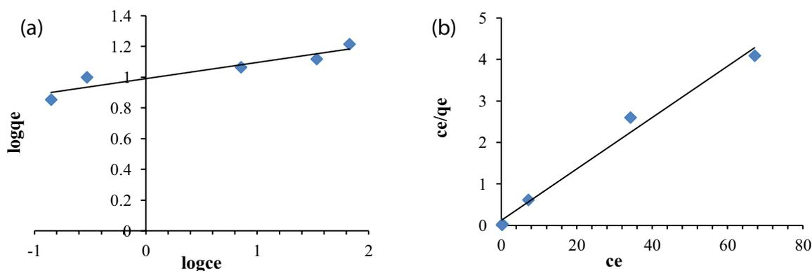
Fig. 9. Adsorption isotherm of MB onto AC, (a) Freundlich adsorption isotherm and (b) Langmuir adsorption isotherm.
