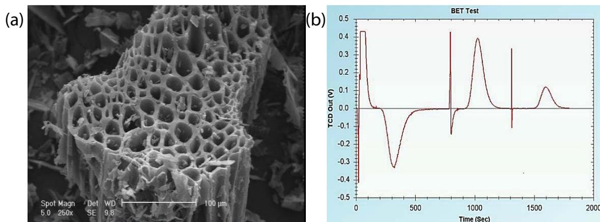
Fig. 2. SEM image (a) and BET test (b) for CSW-AC.
