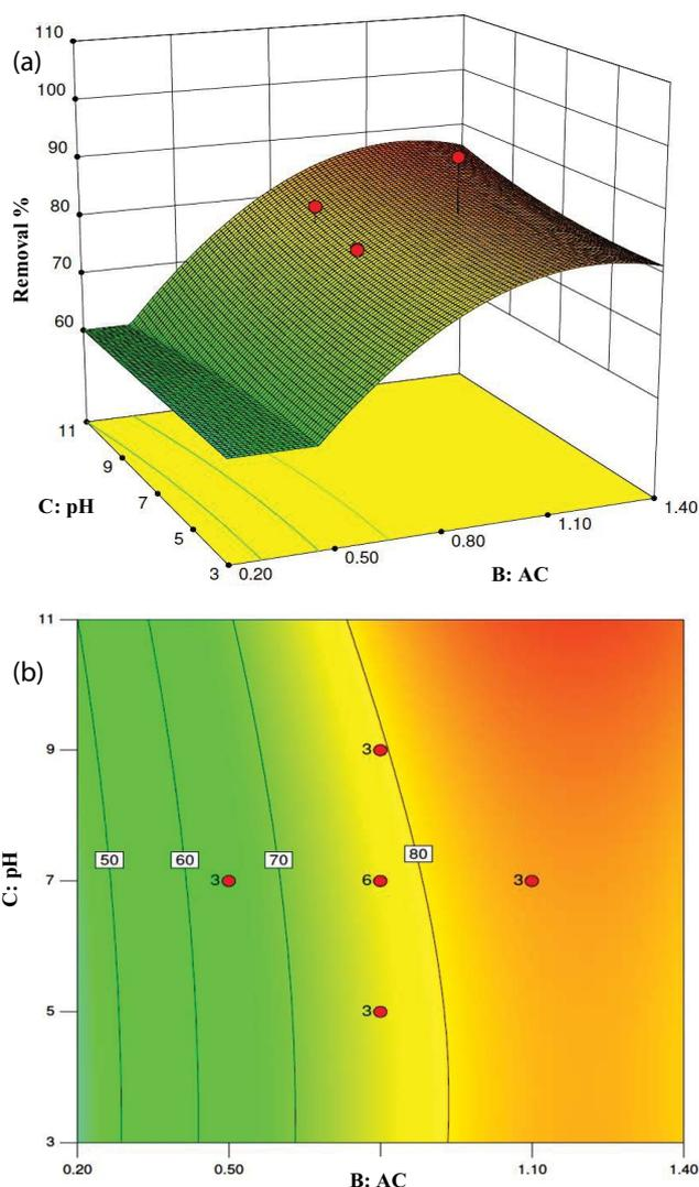
Fig. 5. Response surface plots (a) and response contour plot (b) of pH and AC dosage in the removal of MB (MB = 70 mg/L and contact time = 30 min).
