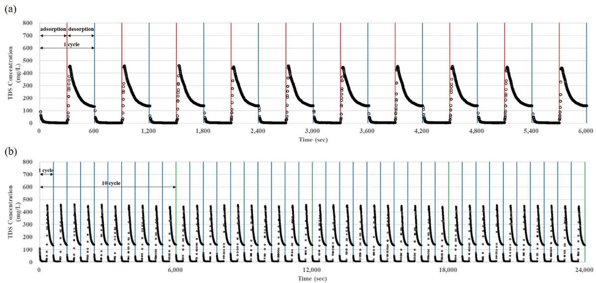
Fig. 4. TDS concentration of adsorption and desorption after (a) 10 cycles and (b) 40 cycles of the MCDI process.
