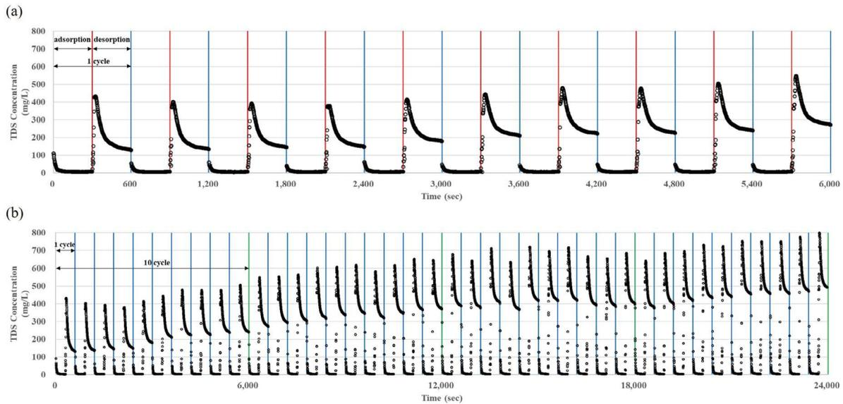
Fig. 5. TDS concentrations of adsorption and desorption after (a) 10 cycles and (b) 40 cycles of the MCDI circulation process.
