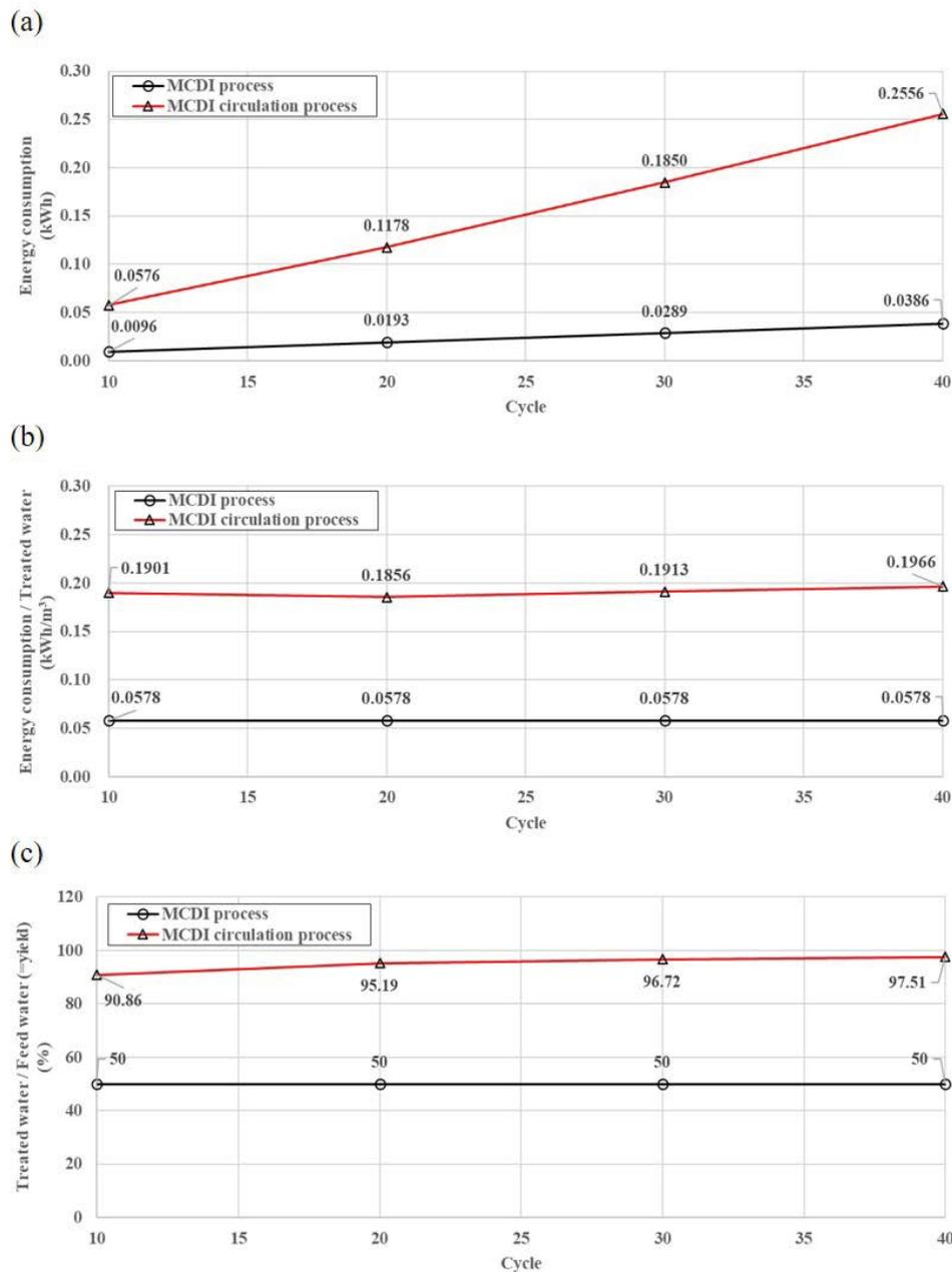
Fig. 7. Comparison of (a) energy consumption, (b) energy consumption per treated water and (c) yield as a function of the number of cycles of the MCDI and MCDI circulation process.
