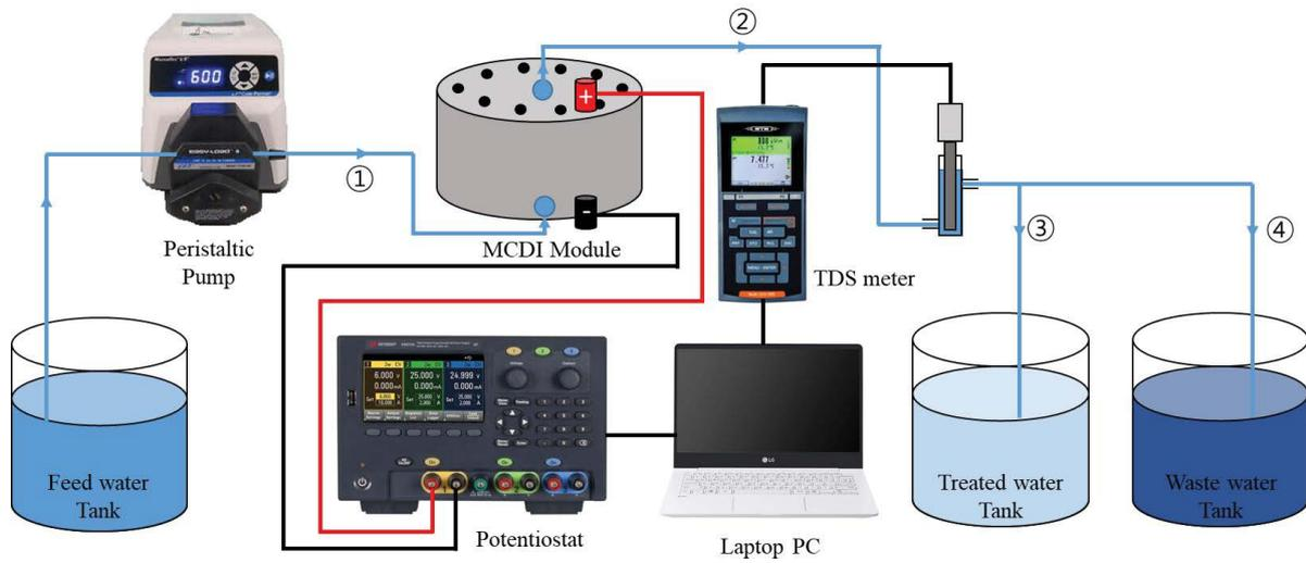
Fig. 2. Schematic diagram of the MCDI process.
