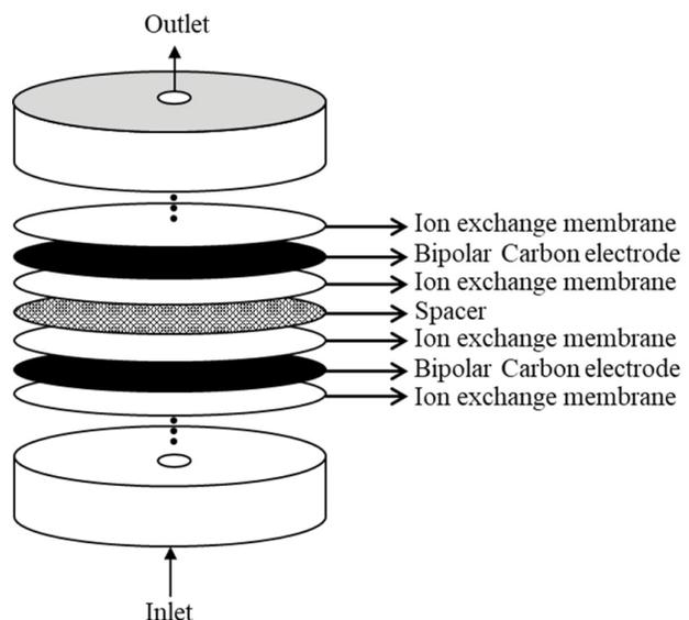
Fig. 1. Configuration schematic of the MCDI module.
