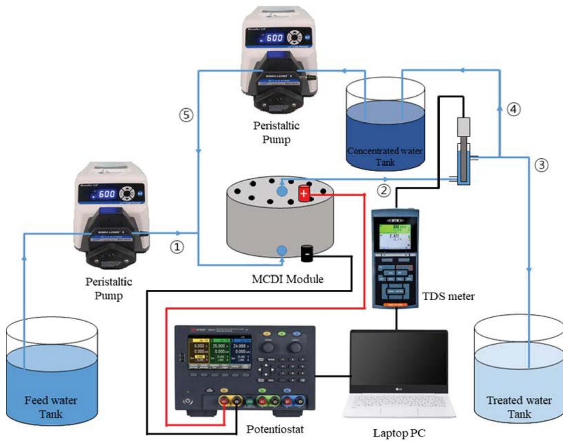
Fig. 3. Schematic diagram of the MCDI circulation process.
