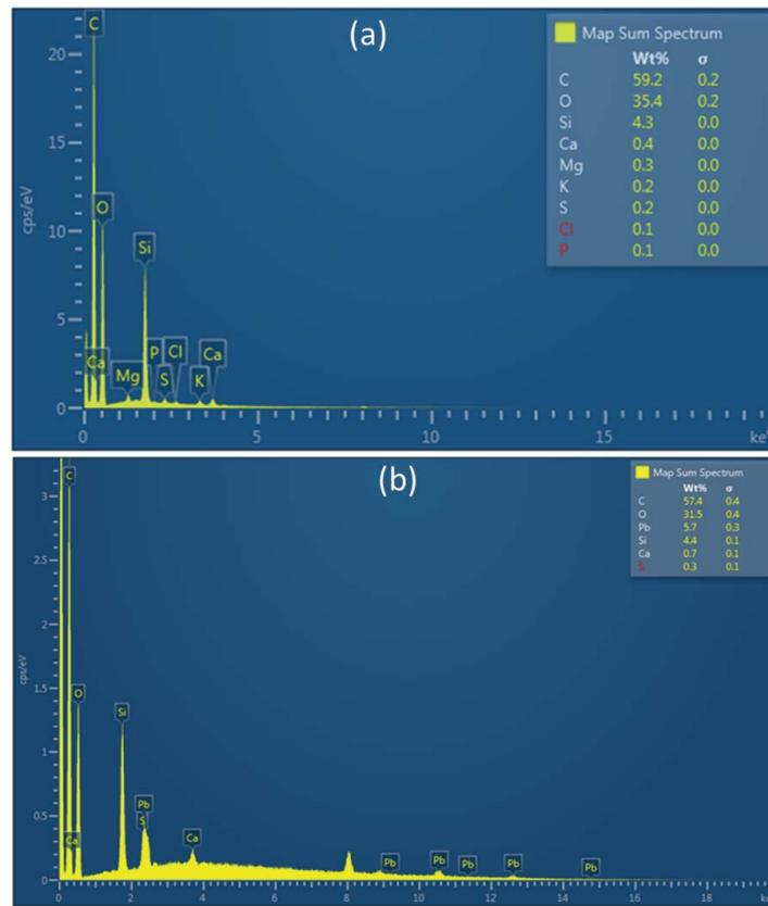
Fig. 4. EDS mapping of palm leaf before (a) and after (b) Pb(II) adsorption.
