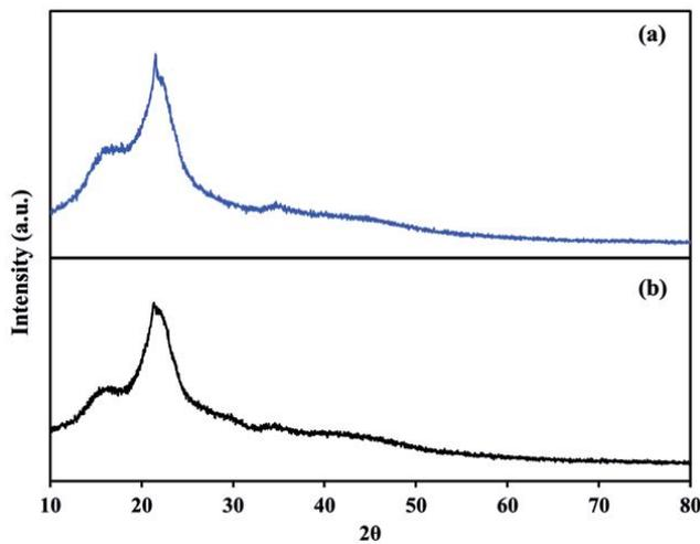
Fig. 6. XRD pattern of palm leaves (a) before and (b) after Pb(II) adsorption.
