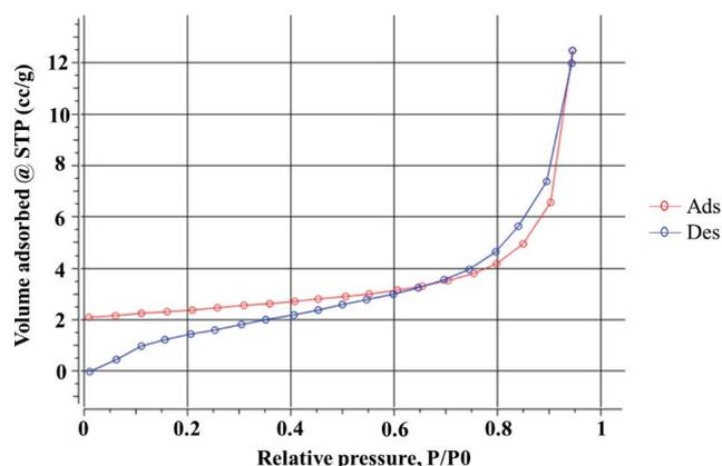
Fig. 2.  $\text{N}_2$  adsorption–desorption isotherm of palm leaves.
