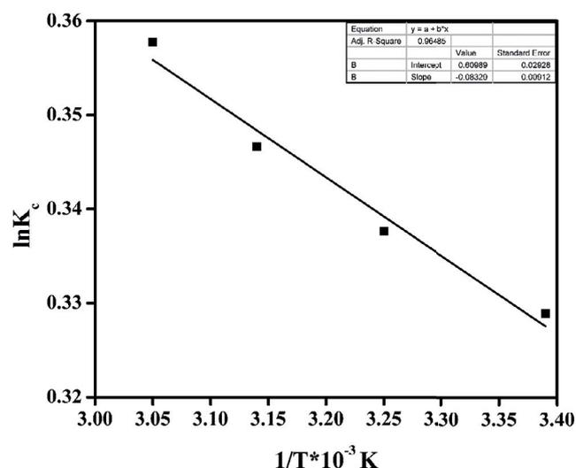
Fig. 11. Plot of  $\ln K_c$  vs.  $1/T$  for Pb(II) adsorption onto palm leaves from an aqueous solution. Temperature 22°C–55°C, initial Pb(II) concentration: 30 mg/L, contact time 1,440 min, initial solution pH 4.8, palm leaves dosage 0.03 g.
