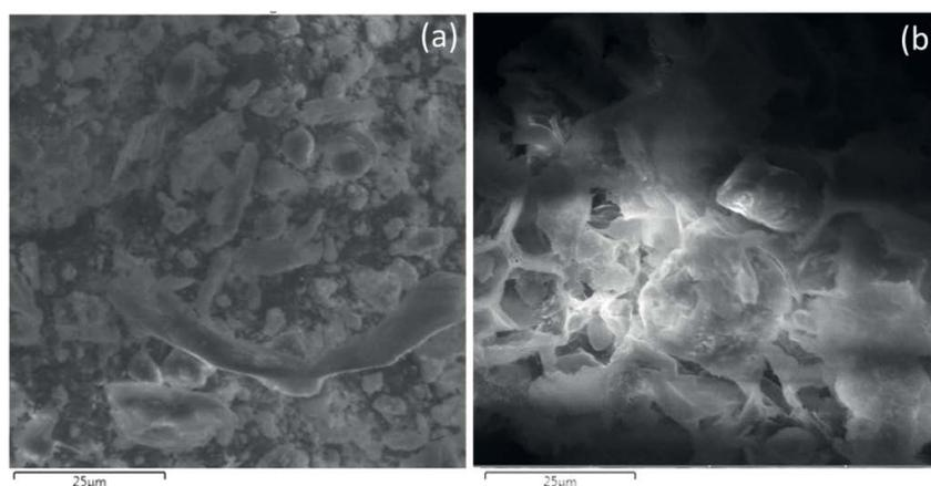
Fig. 3. SEM image of palm leaf (a) before and (b) after Pb(II) adsorption.
