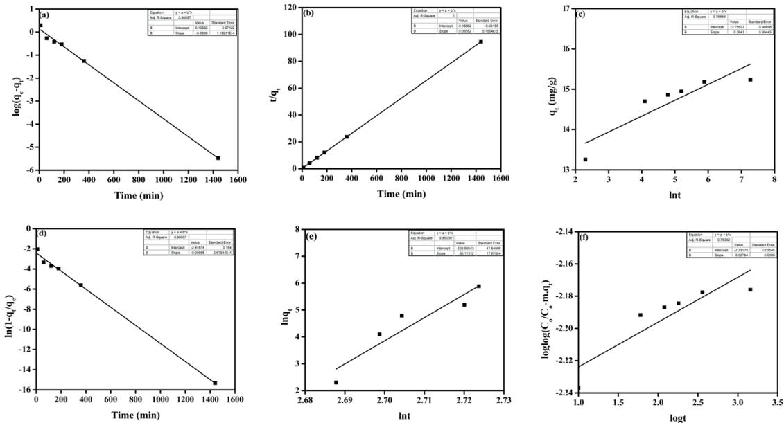
Fig. 9. (a) Pseudo-first-order model, (b) pseudo-second-order model, (c) Elovich model, (d) liquid-film diffusion model, (e) modified Freundlich equation, (f) Bangham equation for Pb(II) adsorption onto palm leaves from aqueous solution. Kinetic experiment conditions: contact time 1–1,440 min, initial Pb(II) concentration: 30 mg/L, temperature: 22°C, initial solution pH 4.8, palm leaves dosage 0.03 g.
