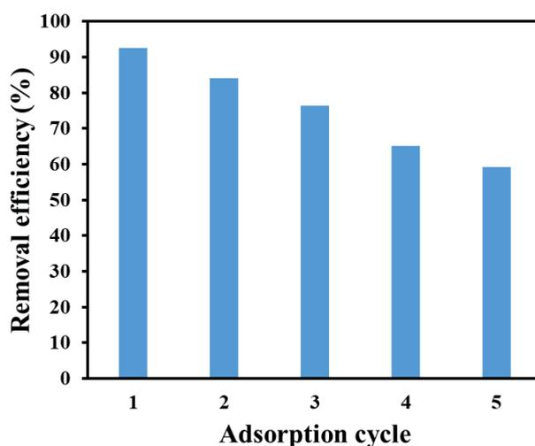
Fig. 12. Removal efficiency of Pb(II) ions onto palm leaves against the number of adsorption/desorption experiments.
