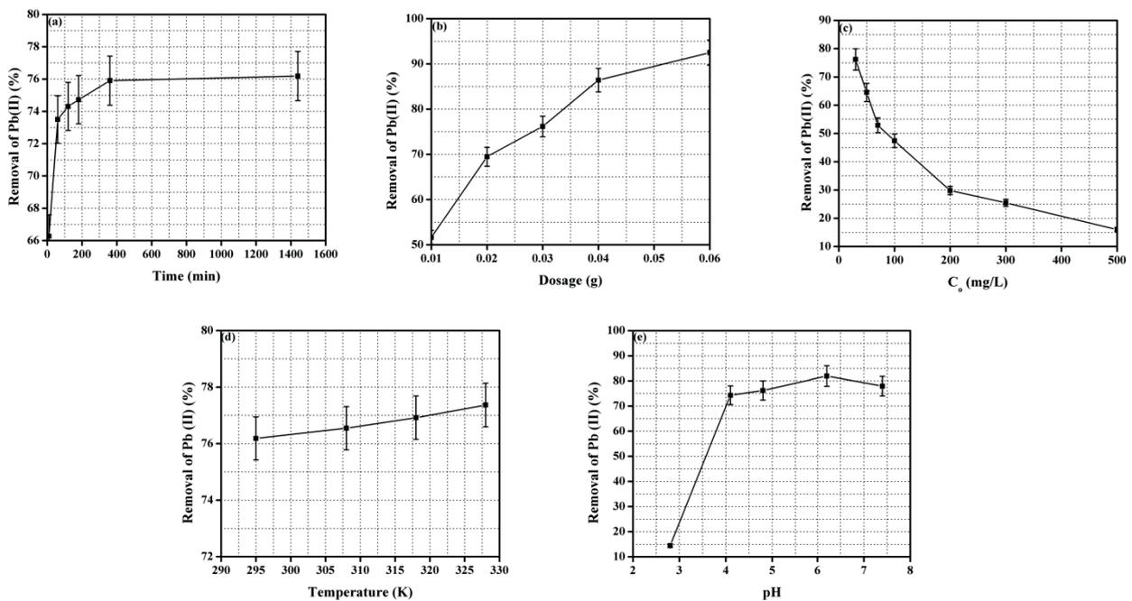
Fig. 7. (a) Effect of contact time, (b) dosage, (c) initial concentration, (d) temperature, (e) pH on the percentage removal of Pb(II) by using palm leaves from an aqueous solution. Sample volume 20 mL, agitation speed 200 rpm. Detailed experimental conditions are provided in Table 1.
