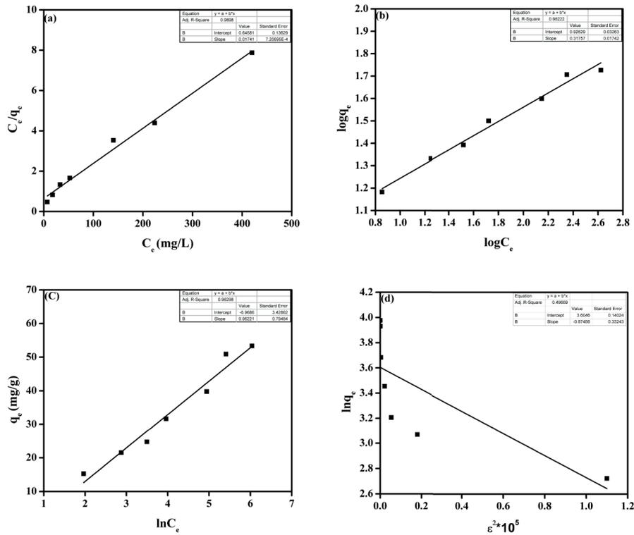
Fig. 10. (a) Langmuir, (b) Freundlich, (c) Temkin, (d) Dubinin–Radushkevich isotherm for Pb(II) adsorption onto palm leaves from an aqueous solution. Isotherm experimental conditions: initial Pb(II) concentration 30–500 mg/L, temperature 22°C, contact time 1,440 min, palm leaves dosage 0.03 g, initial solution pH 4.8.
