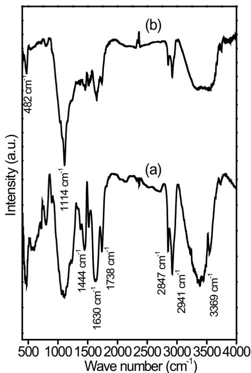
Fig. 5. FTIR spectrum of palm leaves (a) before and (b) after Pb(II) adsorption.
