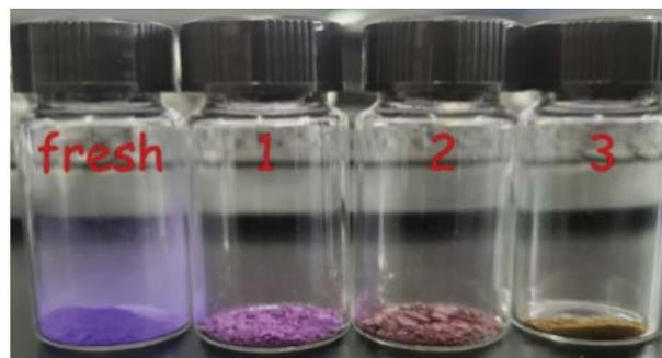
Fig. 3. Photos of the fresh ZIF-67 and after Cr(VI) adsorption for each run.
