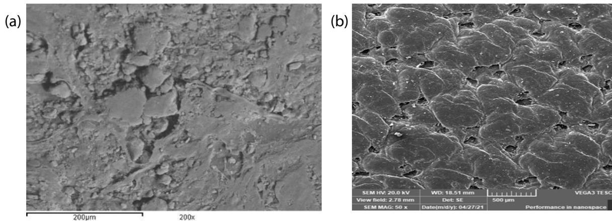
Fig. 4. SEM of grain surface of (a) white shavings (X200) and (b) chromated white shavings (X500).
