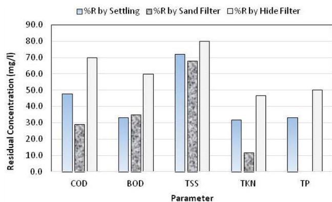
Fig. 7. Efficiency of the combined SF/WSF for the treatment of industrial wastewater.
