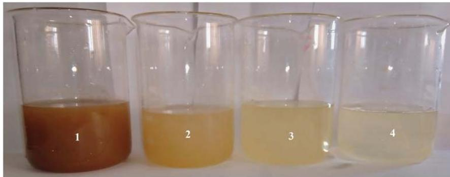
Fig. 6. Treated wastewater (1, raw wastewater, 2, after settling, 3, after sand filter, and 4, the white shavings effluent).
