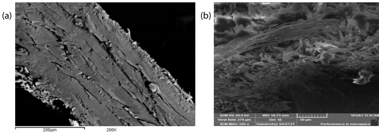
Fig. 5. SEM of cross-section of (a) white shavings (X200) and (b) chromated white shavings (X500).
