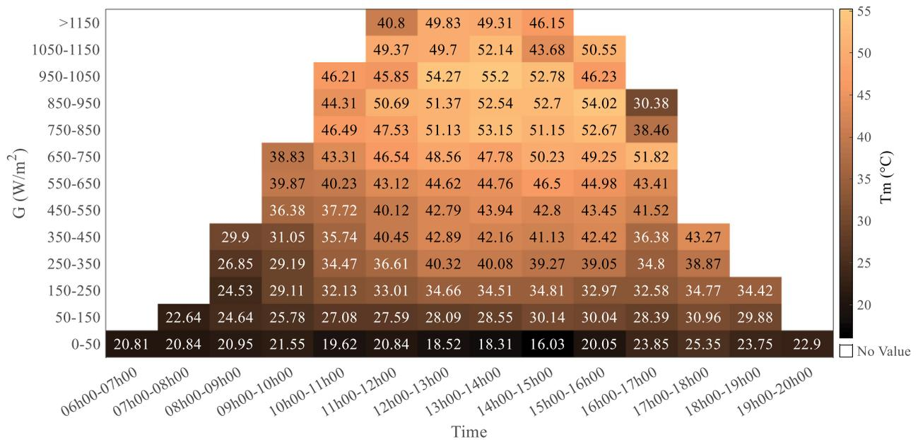
Fig. 8. Tm (°C) vs. G (W/m<sup>2</sup>) and time in 5 months.
