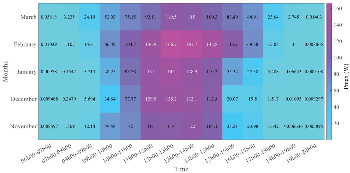
Fig. 5. Evolution of the maximum power supplied over a day in seven (5) months.
