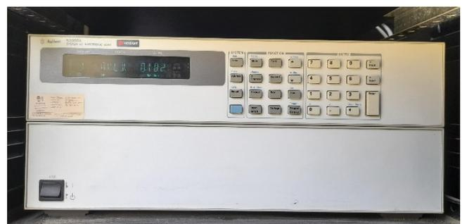
Fig. 3. Electronic charge (Keysight N3300A).
