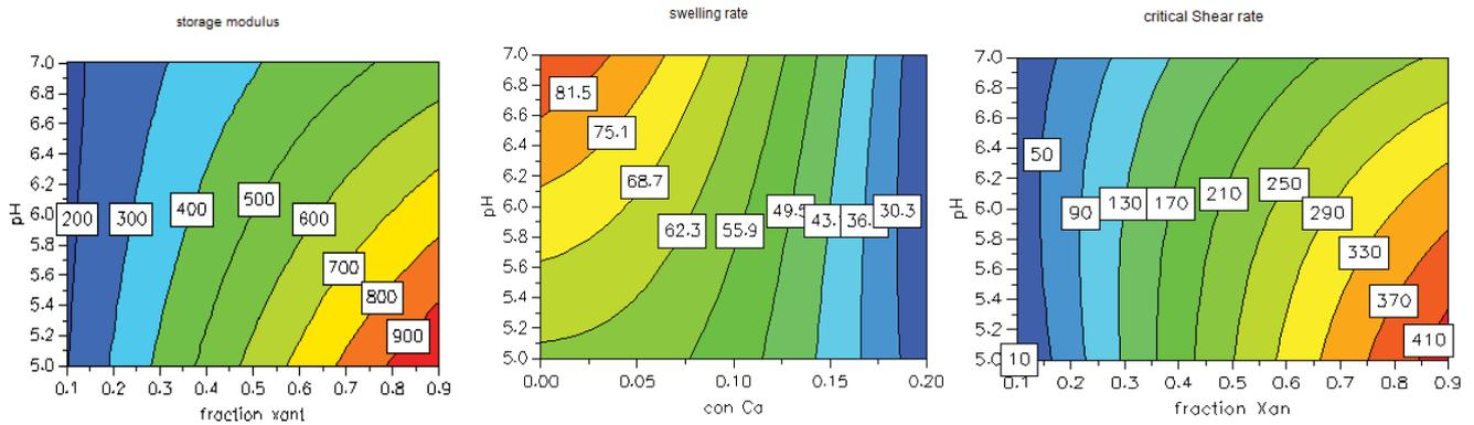
Fig. 4. Isocontours of the three responses, as a function of the variation of the xanthan fraction, concentration of Ca<sup>++</sup> and the pH.
