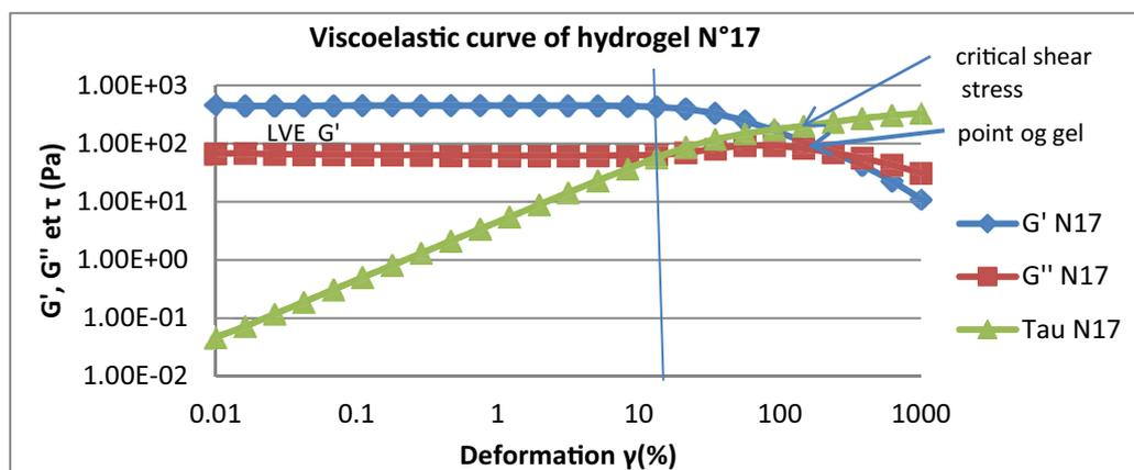
Fig. 1. Viscoelastic behavior of the hydrogel N17.
