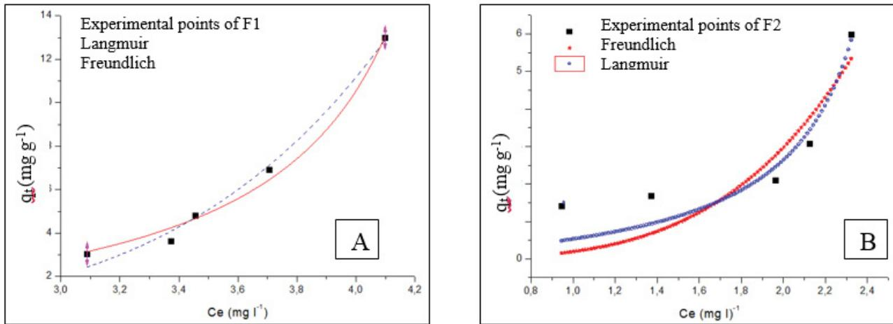
Fig. 9. Modeling of Cd<sup>2+</sup> adsorption isotherm: (A) sample F1 and (B) sample F2.
