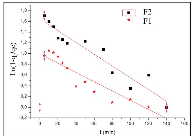
Fig. 8. Modeling plots of intraparticle diffusion of Cd<sup>2+</sup> on beads, using Crank model [30].
