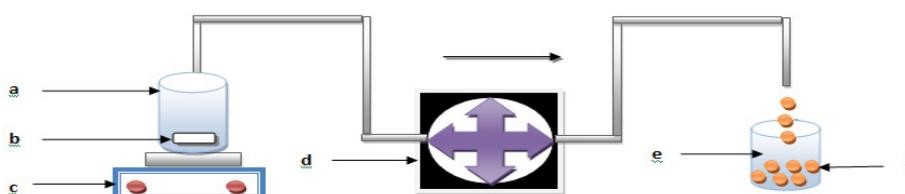
Fig. 2. Diagram of the experimental device illustrating the preparation of the hybrid reinforced porous gelled beads: (a) mixture of (AS/PVA/ $\text{CaCO}_3$ /Al-Mt), (b) magnetic bar, (c) magnetic stirrer, (d) peristaltic pump, (e) solution of  $\text{CaCl}_2$  and boric acid and (f) gelled beads.
