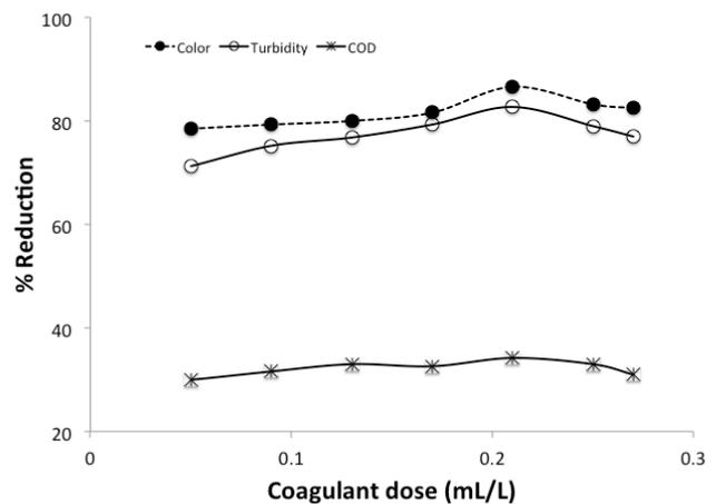
Fig. 2. Percent reductions of color, turbidity and COD in FN nejayote samples. The dose of the coagulant (Sudflock P-63) was varied while the concentration of flocculant (Sumex Biofloc A-01) was maintained at 0.02 mL/L; pH 5.
