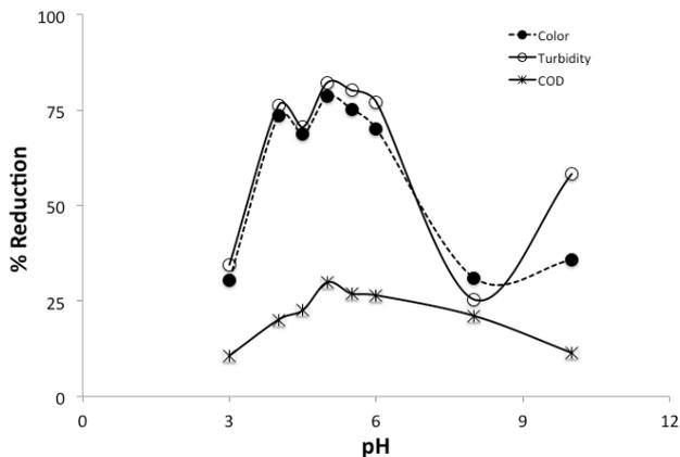
Fig. 1. Percent reductions of color, turbidity and COD in FN nejayote samples as a function of pH with a constant coagulant/flocculant ratio of 2.5.
