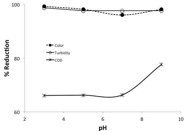
Fig. 3. Percent reductions of color, turbidity and COD in CFN nejayote samples then subjected to electrocoagulation, as a function of pH. Electrolysis conditions: CFN as the nejayote sample, NaCl (5.0 g/L) as the electrolyte, system of Al/Fe electrodes (anode/cathode), potential difference of 9 V, and electrolysis time of 195 min.
