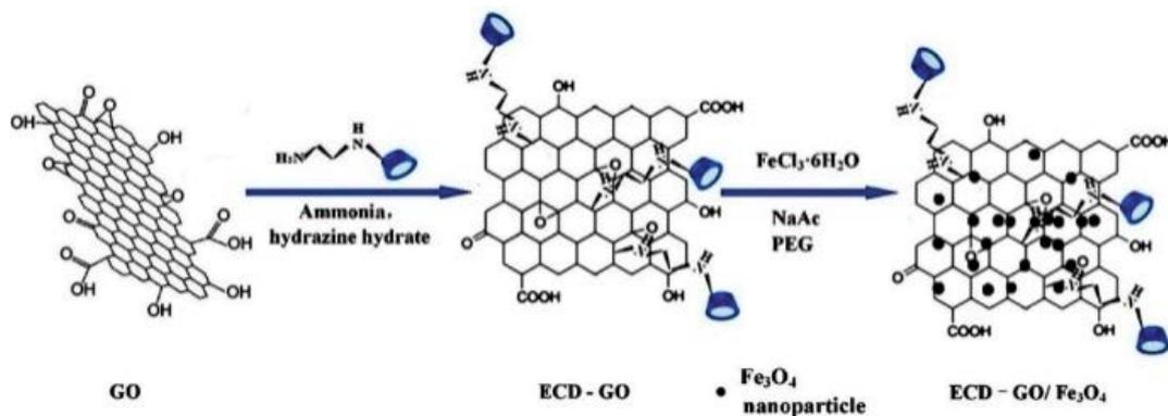
Fig. 1. Illustration of the synthesis process of ECD-GO/ $\text{Fe}_3\text{O}_4$ .
