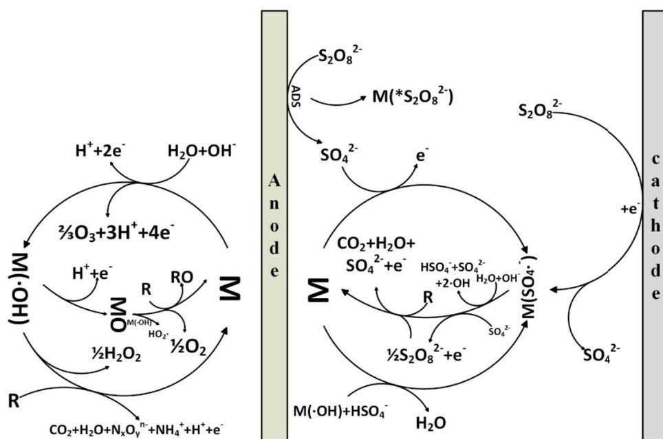
Fig. 1. Mechanism of indirect electro-oxidation of PS and  $H_2O$  (M is anode surface, R is organic matter) [3,23,37,39–43].
