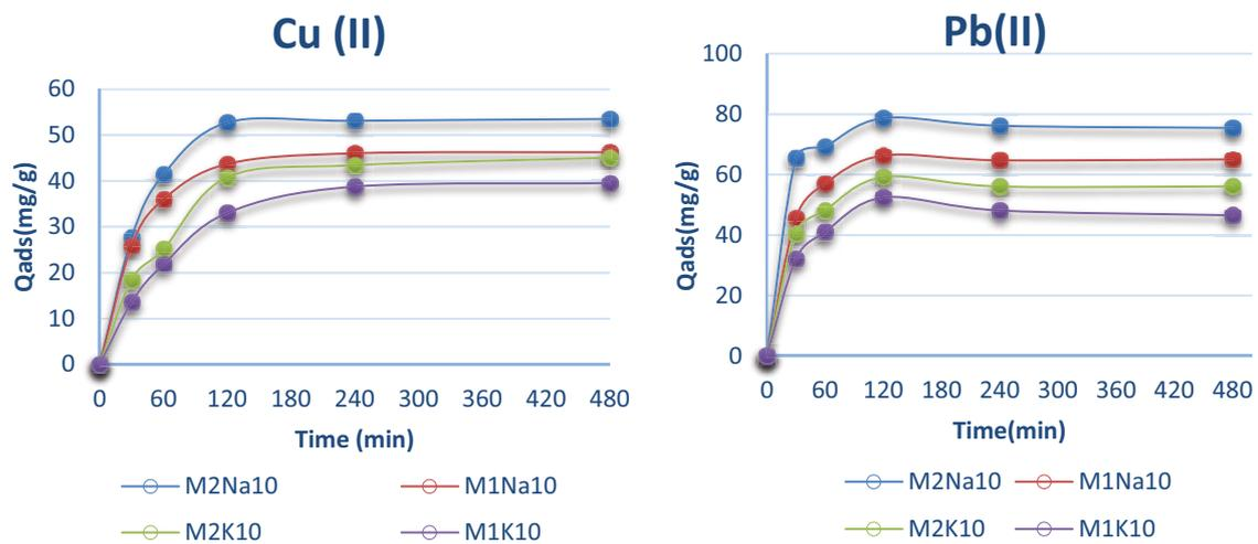
Fig. 7. Effect of contact time on the Cu(II) and Pb(II) adsorption onto geopolymers.
