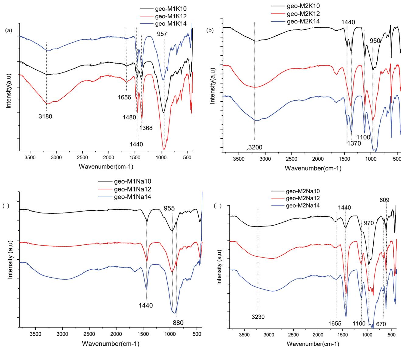
Fig. 5. FTIR spectra of foamed geopolymers (a–d).
