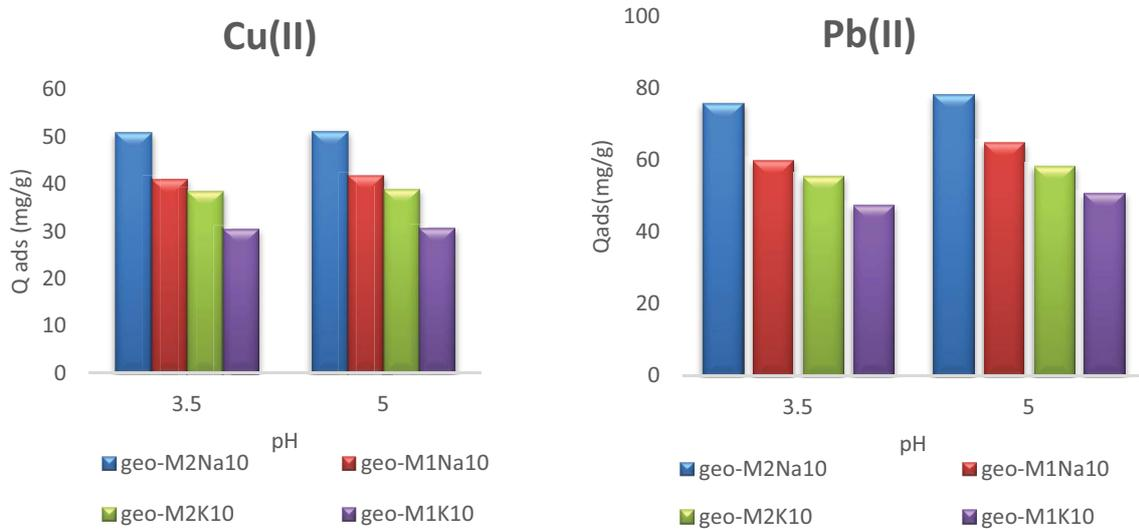
Fig. 6. Effect of pH value on the adsorption process of Cu(II) and Pb(II) onto geopolymers.
