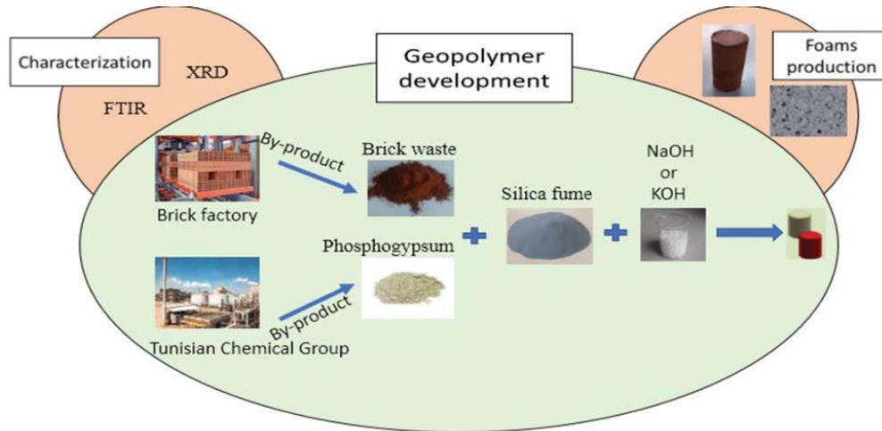
Fig. 1. Synthesis protocol of waste materials based geopolymer.
