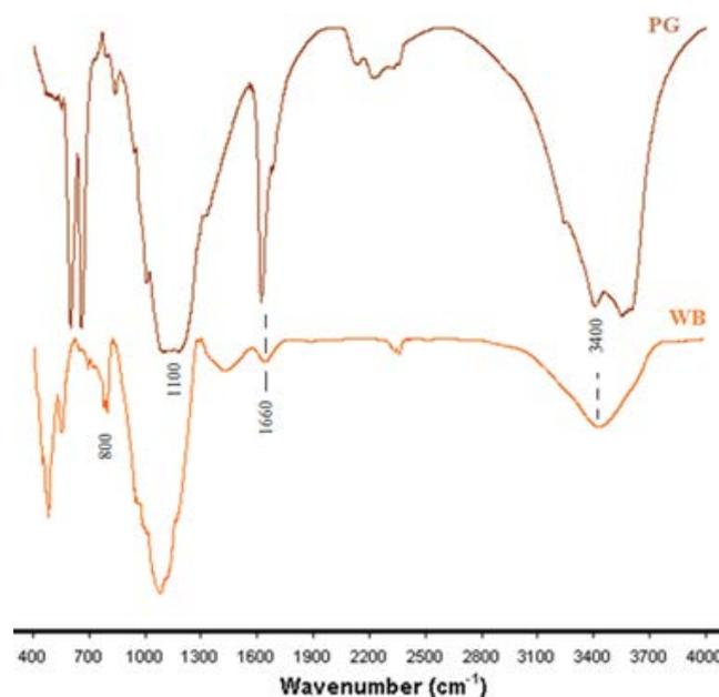
Fig. 3. Infrared spectra of raw materials (PG, WB).
