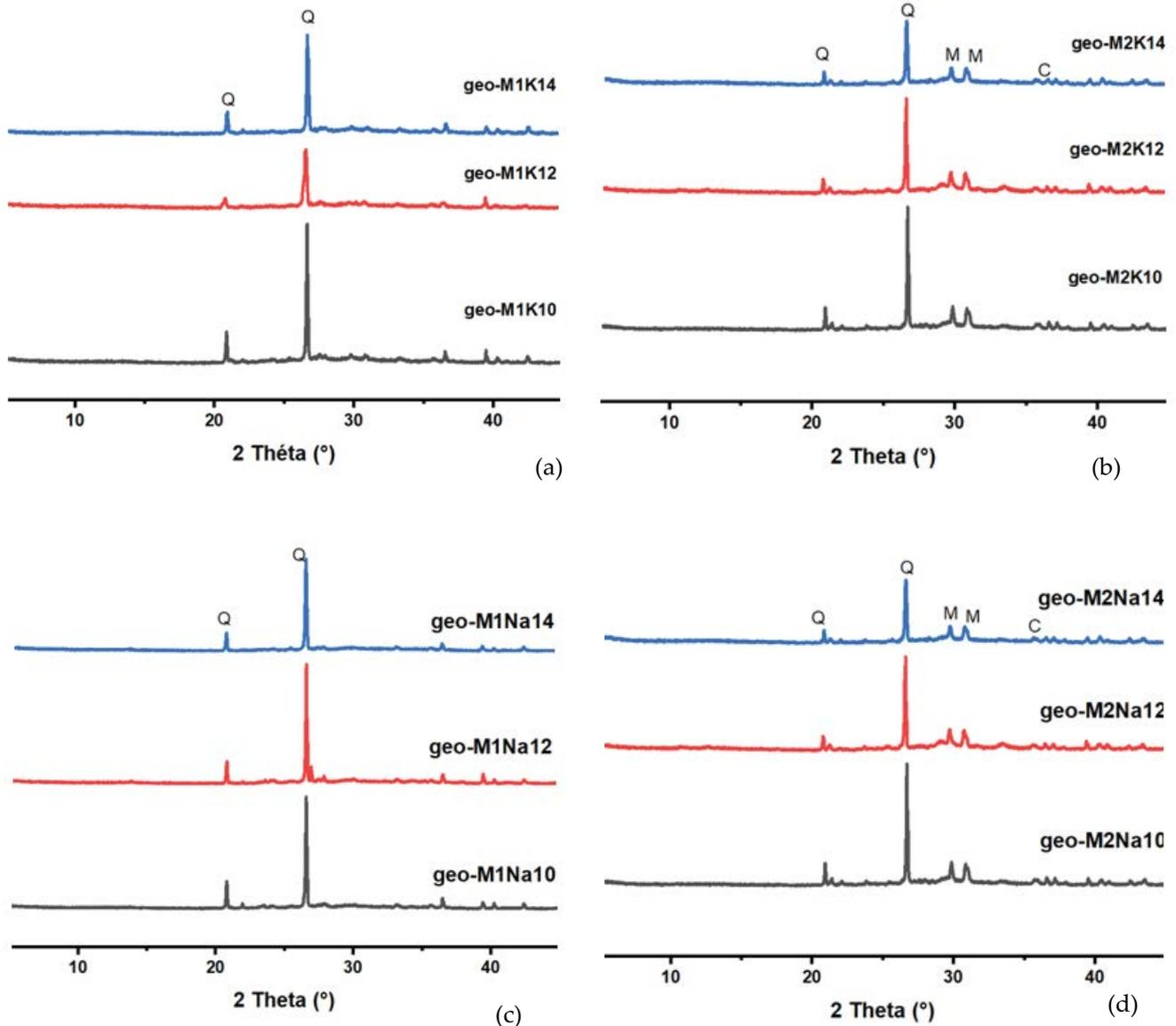
Fig. 4. XRD patterns of foamed geopolymers (a–d). Q: quartz; C: cristobalite; M: mullite.
