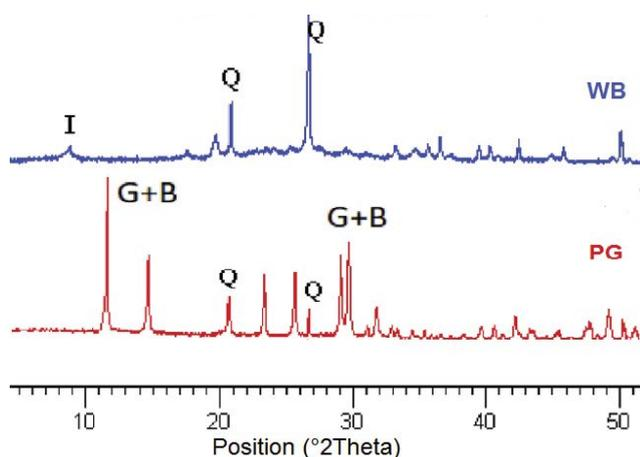
Fig. 2. XRD patterns of raw materials: WB and PG. G: gypsum; B: brushite; Q: quartz; I: illite.
