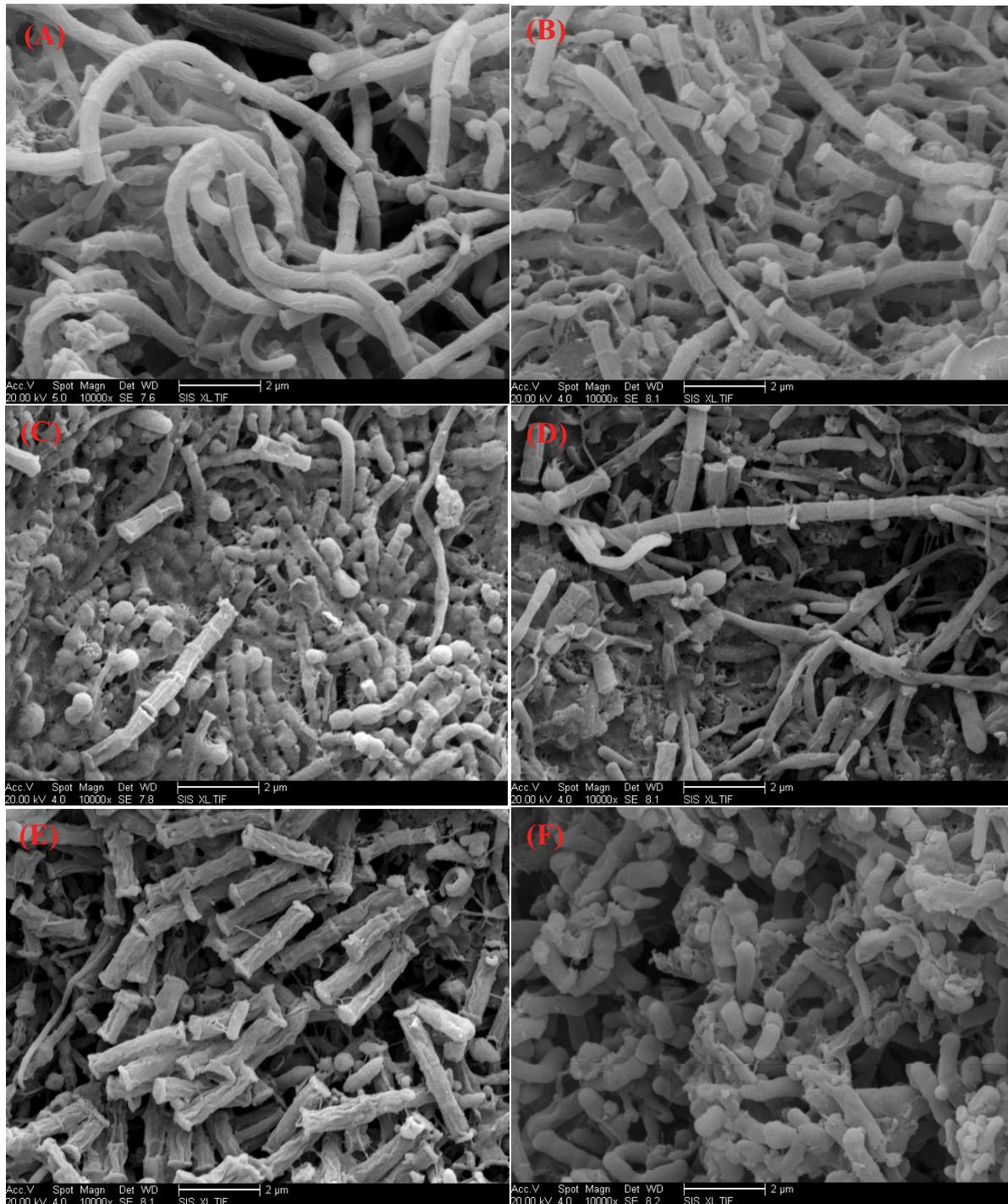
Fig. 5. SEM pictures of anaerobic sludge in EGSB system at different operation stage. (A) Start-up stage (I), (B–E) load increasing stage (II–V) and (F) stable stage (VI). The size bar corresponded to 2  $\mu\text{m}$ .
