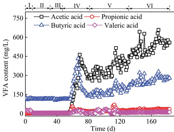
Fig. 3. Changes of VFAs during the start-up and stable stage of EGSB.
