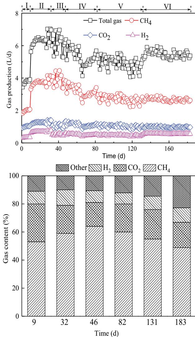
Fig. 4. Changes of daily gas production and gas contents at each stage of EGSB.
