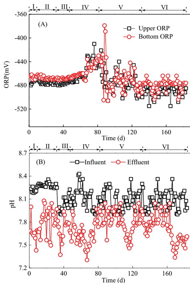
Fig. 1. Changes of ORP and pH with time during the start-up and stable stage of EGSB.
