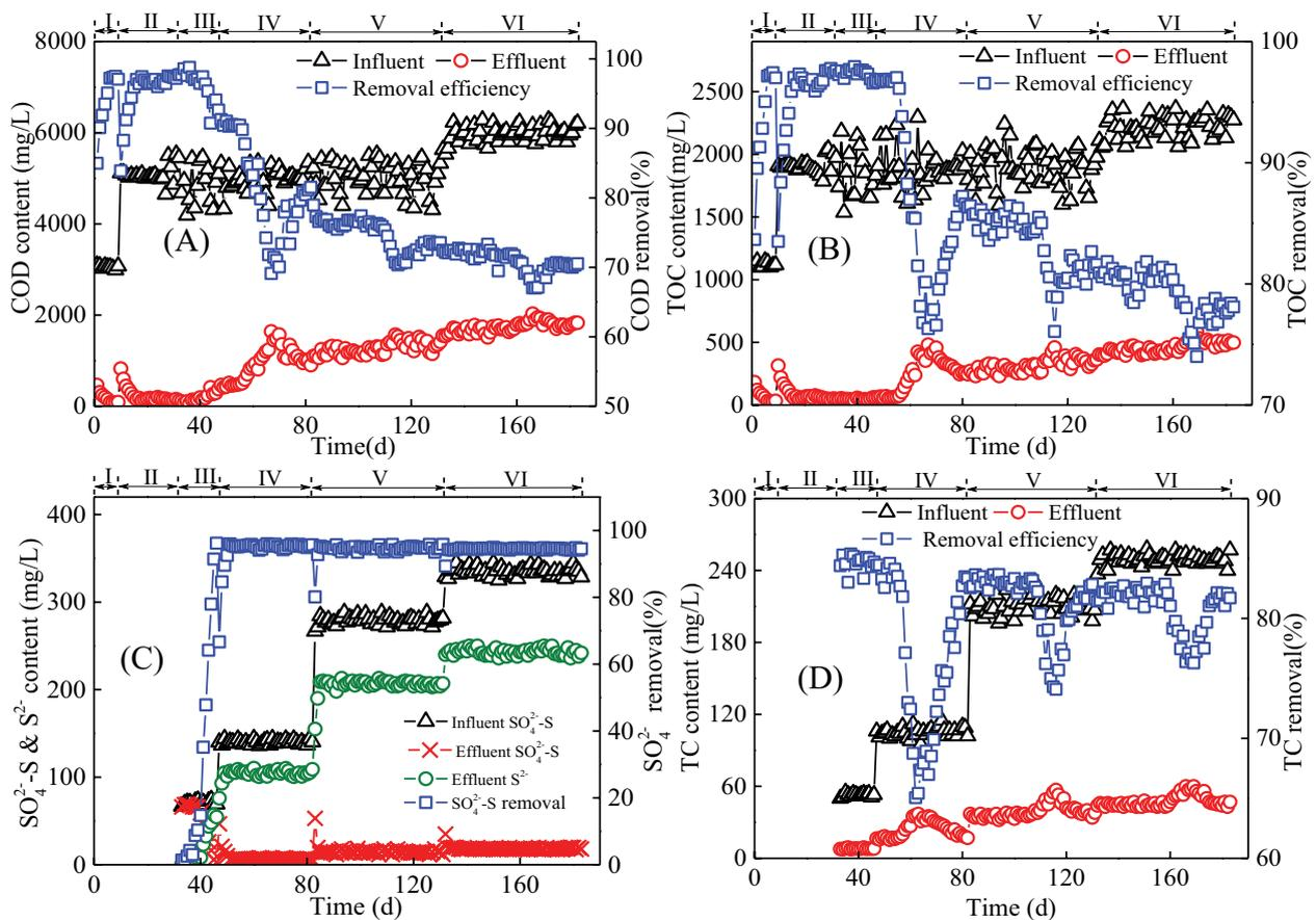
Fig. 2. Changes and removal of various water qualities during the start-up and stable stage of EGSB. (A) COD removal, (B) TOC removal, (C) sulfate removal and sulfide production and (D) TC removal.
