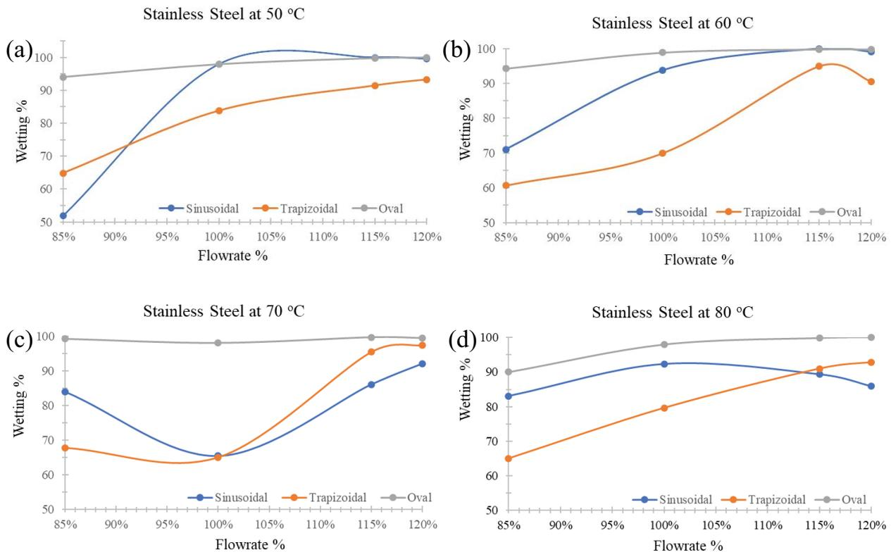
Fig. 4. Wetting % vs. flowrate for stainless steel with different corrugations at temperature different temperatures.
