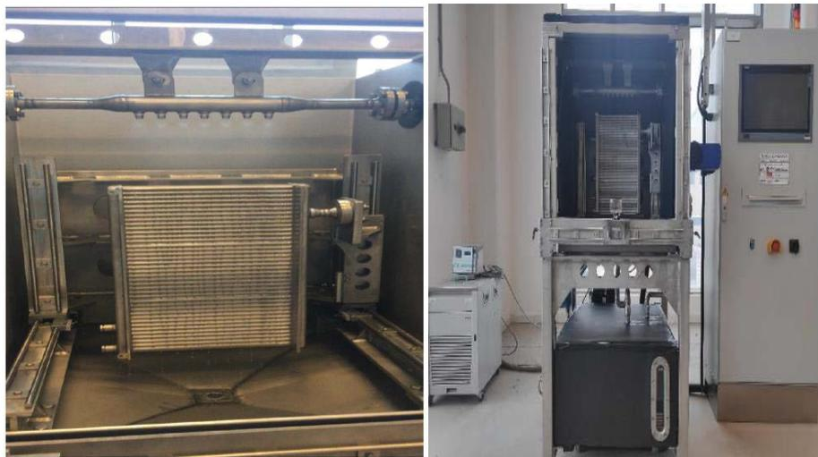
Fig. 2. Hydrodynamic testing unit.
