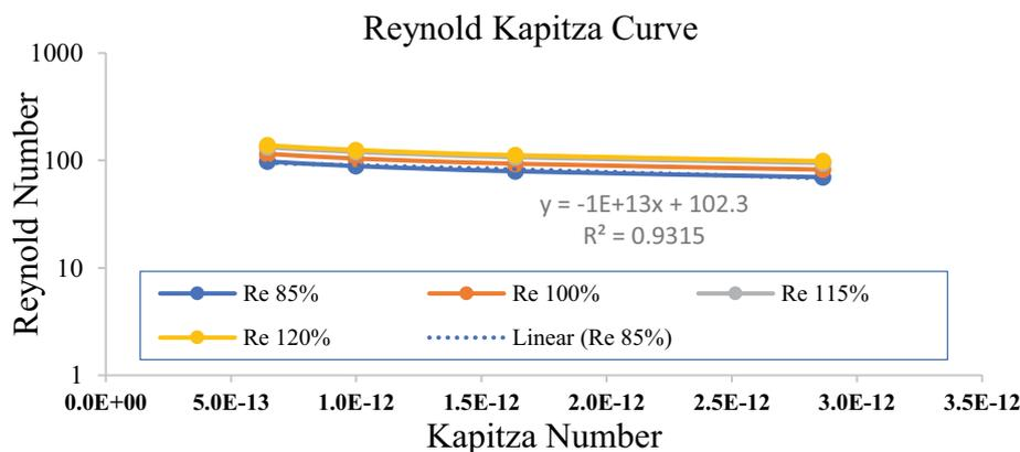
Fig. 3. Re-Ka curve obtained for the 16 points at different flowrates and temperatures.
