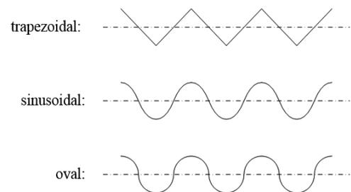
Fig. 1. Schematic view of the three different corrugations.
