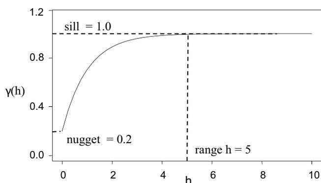
Fig. 2. Description of variogram parameters (sill, range and nuggets).
