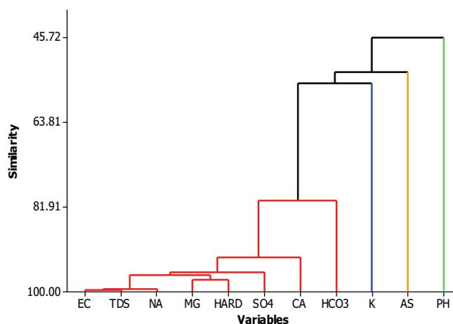
Fig. 3. Dendrogram for clustering the correlated water quality parameters.
