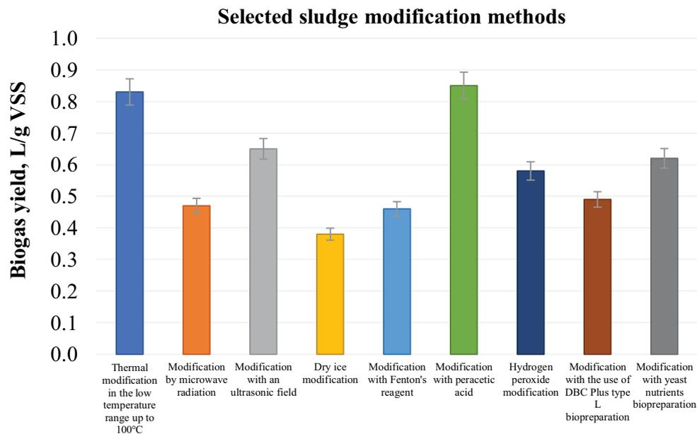
Fig. 6. Biogas yield recorded for the most favorable disintegration conditions.
