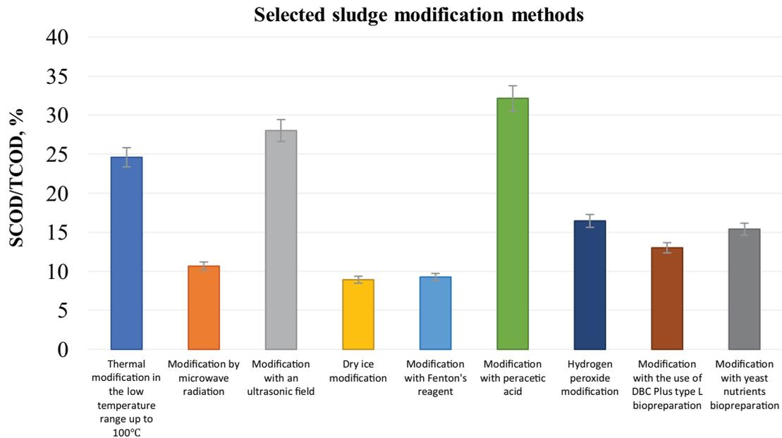
Fig. 5. SCOD/TCOD ratio recorded for the most favorable disintegration conditions.
