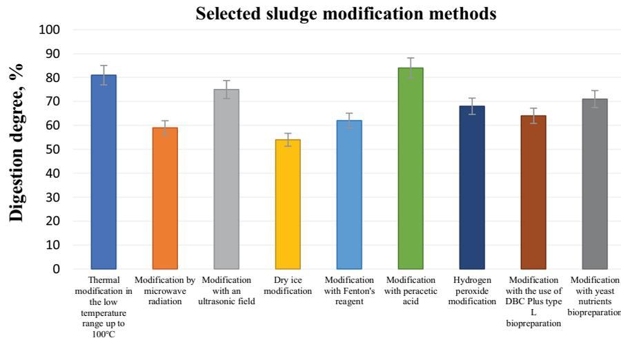
Fig. 7. Digestion degree recorded for the most favorable disintegration conditions.
