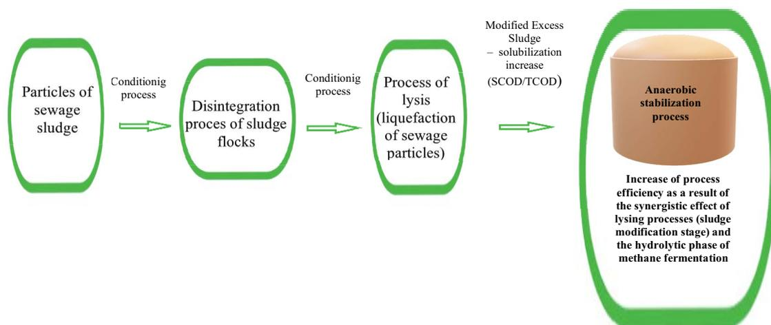
Fig. 1. Idea of the sewage sludge disintegration process (own elaboration on the base of [7]).
