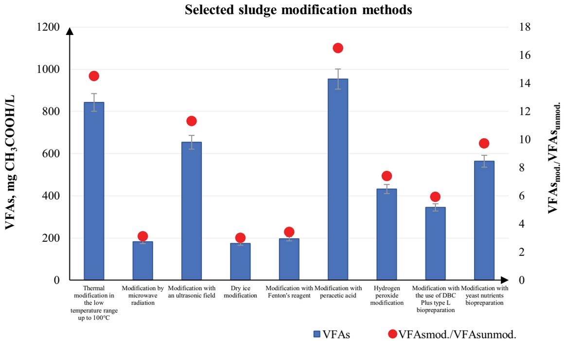
Fig. 4. Volatile fatty acids concentration recorded for the most favorable disintegration conditions.
