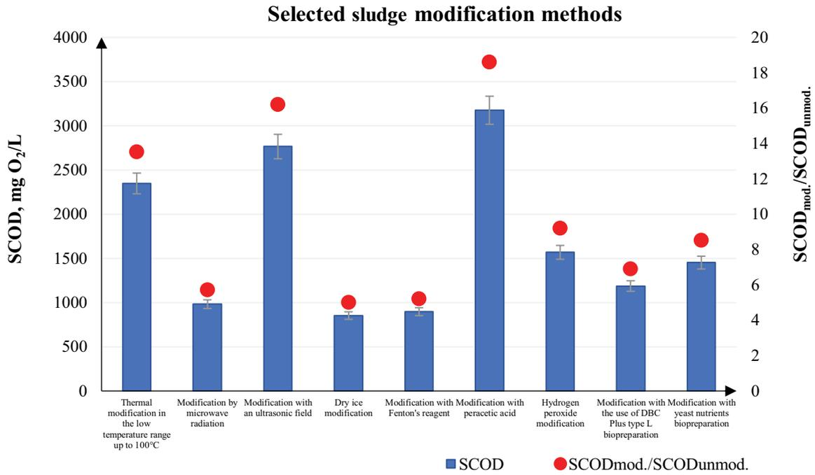
Fig. 3. SCOD value recorded for the most favorable disintegration conditions.
