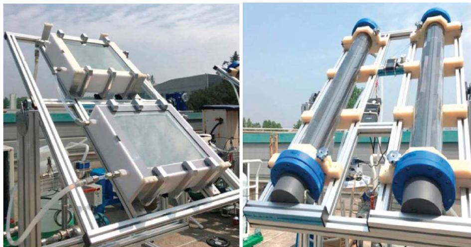
Fig. 5. Photographs of photocatalytic scale-up reactors including  $\text{TiO}_2$  (a) flat-type reactor (b) rotating-type reactor (compiled from [129,130]).
