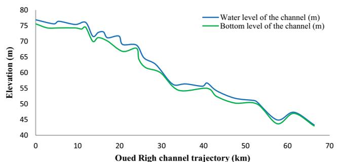
Fig. 9. Longitudinal section of Oued Righ channel (April).
