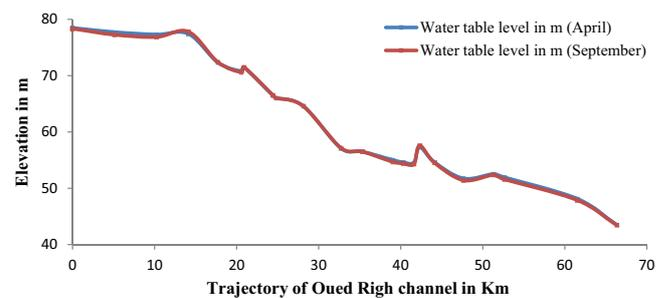
Fig. 8. Piezometric profile of phreatic water.
