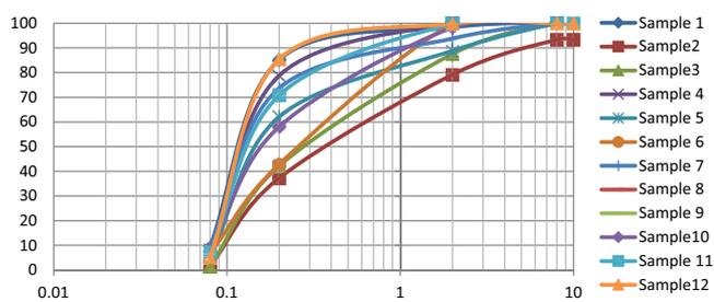
Fig. 13. Grain size distribution curves of analysed sediments.
