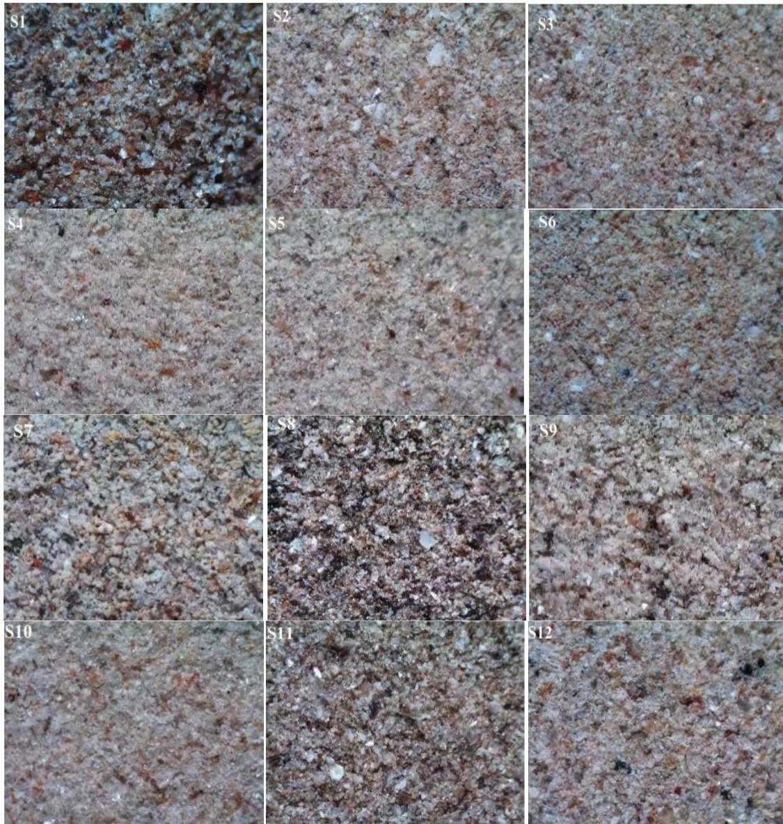
Fig. 12. Microscopy images of sediment samples.
