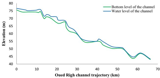
Fig. 10. Longitudinal section of Oued Righ channel (September).
