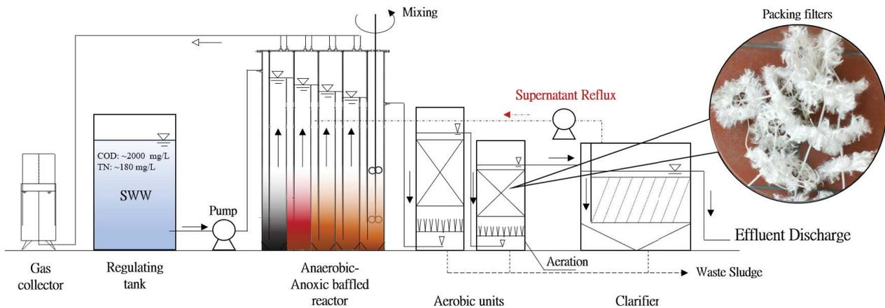
Fig. 1. Flowchart of upgraded anaerobic-aerobic slaughterhouse wastewater treatment process (U-AASWWTP).
