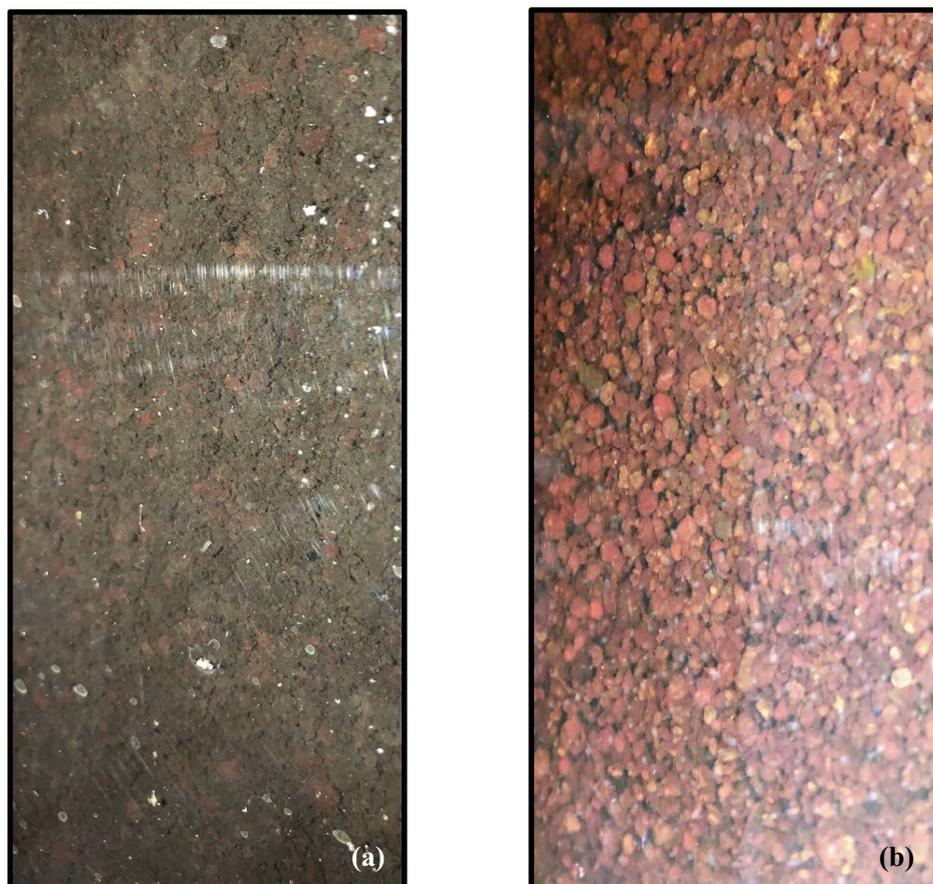
Fig. 3. Pictures of reddish-brown microbial granular sludge formation process in A-ABR. (a) Picture of 3A bottom on the 68th day of run and (b) picture of 2A bottom on the 300th day of run.
