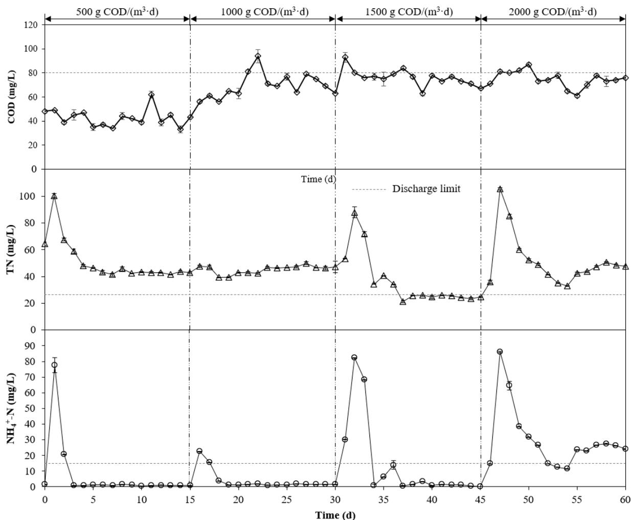
Fig. 5. Effluent COD, TN, and  $\text{NH}_4^+\text{-N}$  concentrations from U-AASWWTP at the different organic loading rates.
