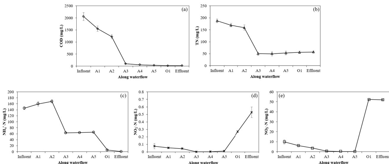
Fig. 2. Profiles of COD, TN,  $\text{NH}_4^+\text{-N}$ ,  $\text{NO}_2^-\text{-N}$ , and  $\text{NO}_3^-\text{-N}$  concentrations vs. waterflow from influent to effluent in central points of BBD for U-AASWWTP.
