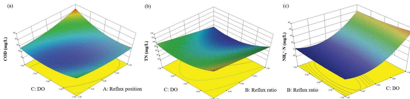
Fig. 4. Interaction between independent variables in U-AASWWTP shown on 3D surface plots. (a) Reflux position and dissolved oxygen of effluent COD, (b) reflux ratio and dissolved oxygen of effluent TN and (c) reflux ratio and dissolved oxygen of effluent  $\text{NH}_4\text{-N}$ .
