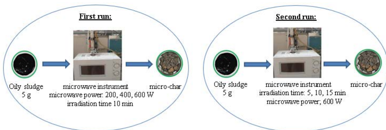
Fig. 1. Schematic illustration microwave process of oily sludge to micro-char production.
