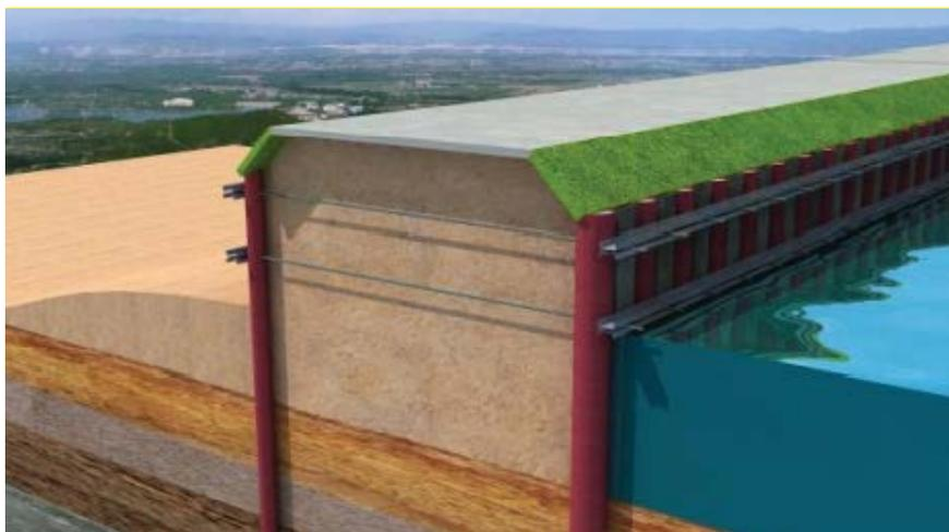
Fig. 4. Schematic diagram of PC combined method pile cofferdam.
